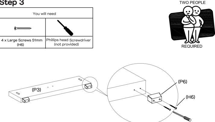
Attach footboard leg (P6) to the bottom of footboard (P3) with 4 x Large Screw 51mm (H6) by using phillips head screwdriver (not provided).
