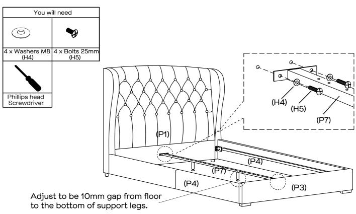
Slot the centre raill (P7) into the headboard (P1) and footboard (P3) Rotate bolts (H5) by using phillips head screwdriver (not provided) to the headboard (P1) and footboard (P3). No need to tighten bolts until step 8.
