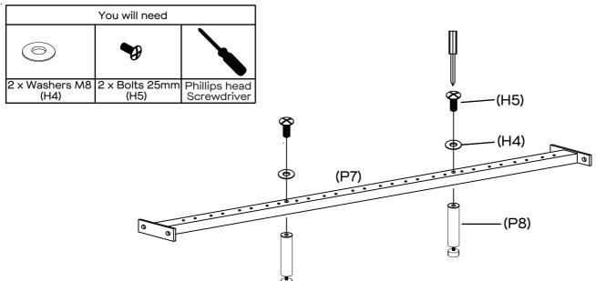
Attach the support legs (P8) to the centre rail (P7) using  $2 \times Bolts$  (H5),  $2 \times Washers$  (H4) as shown.
