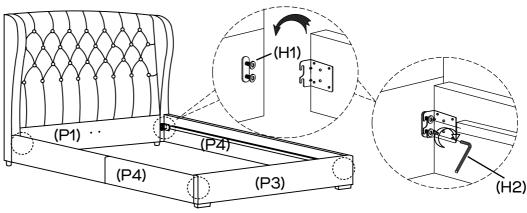
Install the bolts (H1) to the brackets by using Allen key (H2) as shown, do not tighten the bolts and keep them 8 mm loose. Then attach side rails (P4) to headboard (P1) and footboard (P3) by slotting the bracket on the side rails (P4) over the bolt as shown. No need to tighten bolts until step 8.
