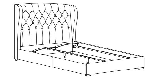
Insert the full slat into the side rail and centre rail one by one.
