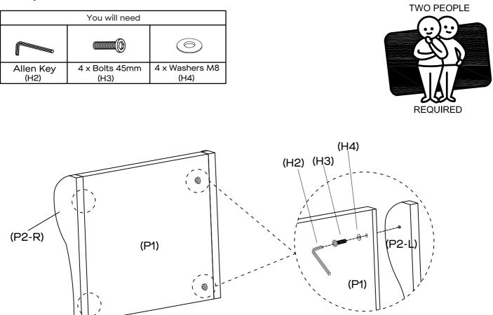
Attach Wing (P2-L;P2-R) to the headboard (P1) with 4 x washers (H4) and 4 x Bolt 45mm (H3) by using Allen key (H2) as shown.
