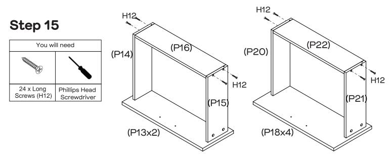
Attach Drawer Back (P16x2) to Left & Right Drawer Sides (P14x2 & P15x2) with 8 x Long Screws (H12) by tightening with the Phillips Head Screwdriver. Attach Drawer Back (P22x4) to Left & Right Drawer Sides (P20x4& P21x4) with 16 x Long Screws (H12) by tightening with the Phillips Head Screwdriver. Before securing - Ensure the Bottom Panel lines up with the grooves the whole way around the drawer.
