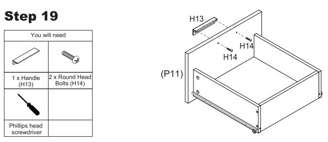
Attach 1 x Handle (H13) to Drawer Front (P11) with 2 x Round Head Bolts (H14). Tighten round head bolts using a Phillips head screwdriver. Repeat Step 14 to Step 19 to assemble the other drawer.
