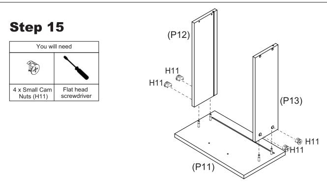
Insert 4 x Small Cam Nuts (H11) into the holes of Drawer Sides (P12, P13). Rotate the cam nuts so the arrows point towards the incoming cam bolts. Align the holes together, secure Drawer Sides (P12, P13) into place and tighten the cam nuts using a Flat head screwdriver.
