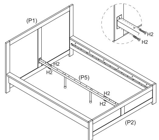
Attach Centre Rail (P5) to Bedhead (P1) and Bedfoot (P2) as shown. Then screw Centre Rail (P5) with 4 x Screws (H2).
