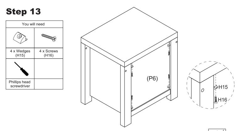
Secure Back Panel (P6) in place with 4 x Wedges (H15) using 4 x Screws (H16). www.fantasticfurniture.com.au
