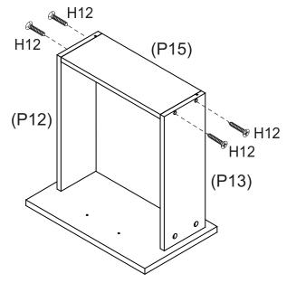
Attach Drawer Back (P15) to Drawer Sides (P12, P13) with 4 x Long Screws (H12), make sure that the groove lines up the whole way around the drawer. Tighten Screws using a Phillips head screwdriver.
