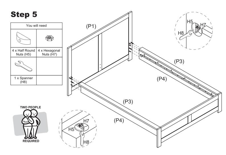
Attach Bedhead (P1) to Side Covers (P3) and Side Rails (P4) with 4 x Half Round Nuts (H5) and 4 x Hexagonal Nuts (H7) using Spanner (H8).
