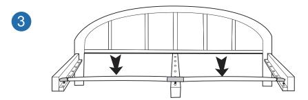
Sometimes it makes it easier to line up the hole if you press down in the middle of the slat to flatten it out.
