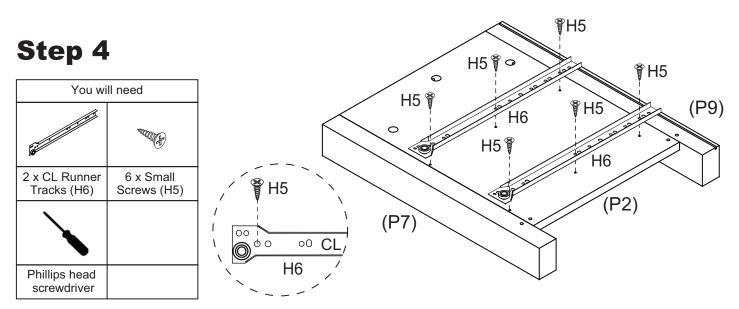
Attach 2 x CL Runner Tracks (H6) to Left Side Panel (P2) with 6 x Small Screws (H5).
