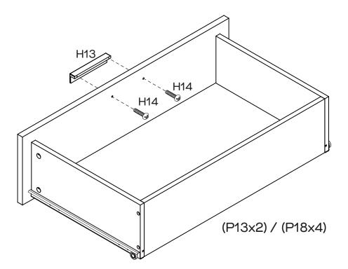
Attach 6 x Handles (H13) to Drawer Fronts (P13x2, P18x4) with 12 x Handle Bolts (H14). Tighten Round Head Bolts using a Phillips head screwdriver.
