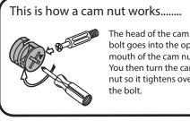
The head of the cam bolt goes into the open mouth of the cam nut. You then turn the cam nut so it tightens over
