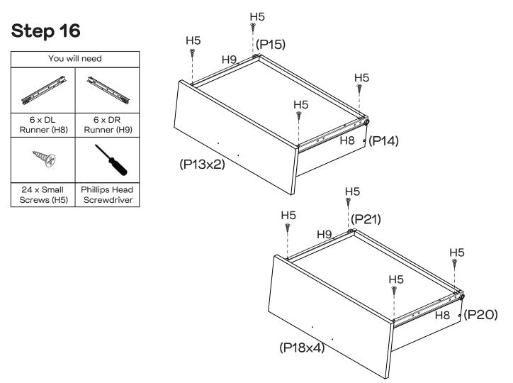
Attach 6 x DL Runner (H8) to Left Drawer Side (P14x2 & P20x4) and 6 x DR Runner (H9) to Right Drawer Side (P15x2 & P21x4) with 24 x Small Screws (H5) by tightening with the Phillips Head Screwdriver.
