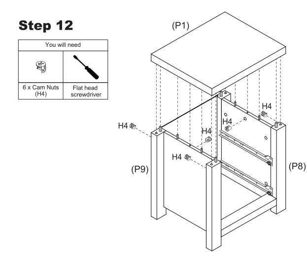
Insert 6 x Cam Nuts (H4) into the holes of Side Panels (P2, P3) and Legs (P7, P8, P9, P10). Rotate the cam nuts so the arrows point towards the incoming cam bolts. Attach Top Panel (P1) to the frame and tighten the cam nuts using a Flat head screwdriver.
