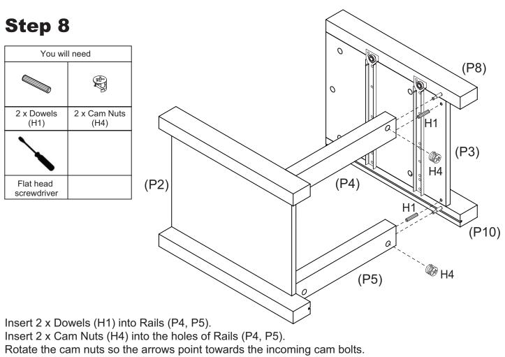
Align the holes and attach Legs (P8, P10) to Right Side Panel (P3). Tighten the cam nuts.
