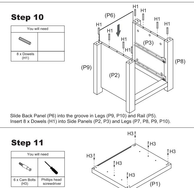
Attach 6 x Cam Bolts (H3) into Top Panel (P1) as shown.
