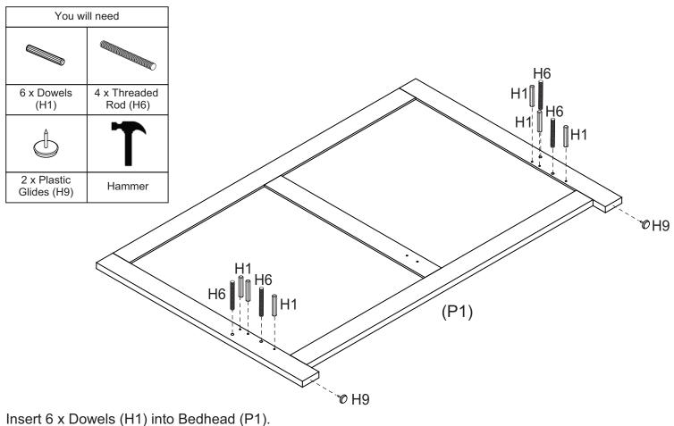
Attach 4 x Threaded Rod (H6) into Bedhead (P1). Hammer 2 x Plastic Glides (H9) onto the bottom of Bedhead (P1).
