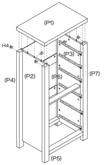
Insert 6 x Cam Nuts (H4) into the holes of Side Panels (P2, P3) and Legs (P4, P5, P6, P7). Rotate the cam nuts so the arrows point towards the incoming cam bolts. Attach Top Panel (P1) into place, and then tighten the cam nuts.
