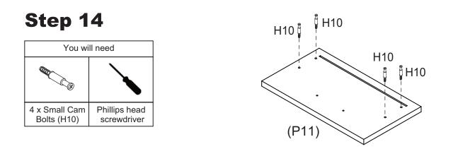
Screw 4 x Small Cam Bolts (H10) into Drawer Front (P11) with a Phillips head screwdriver.
