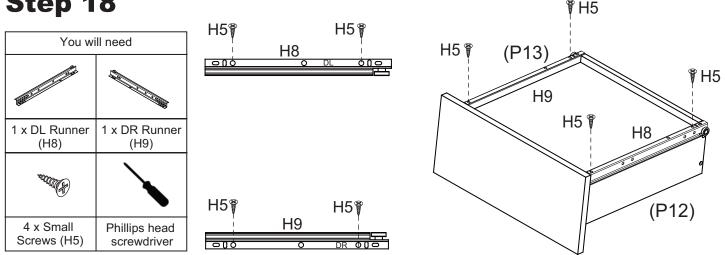
Attach 1 x DL Runner (H8) to the bottom of Left Drawer Side (P12) and 1 x DR Runner (H9) to the bottom of Right Drawer Side (P13) with 4 x Small Screws (H5). Tighten Screws using a Phillips head screwdriver.
