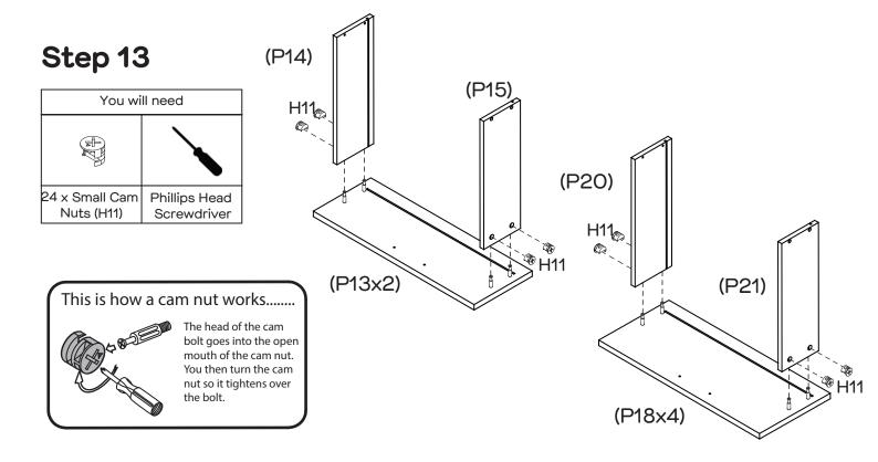
Insert 24 x Small Cam Nuts (H11) into Left Drawer Sides (P14x2 & P20x4) & Right Drawer Sides (P15x2 & P21x4), attach to Drawer Fronts (P13x2, P18x4) by tightening Cam Nuts with the Phillips Head Screwdriver.
