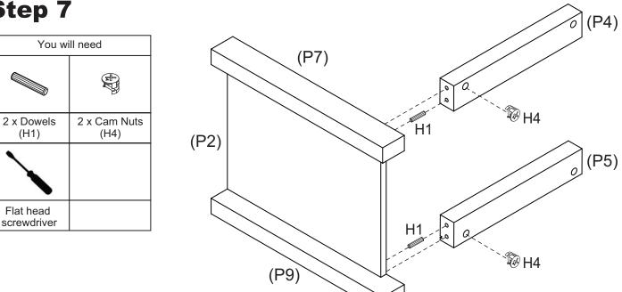
Insert 2 x Dowels (H1) into Rails (P4, P5). Insert 2 x Cam Nuts (H4) into the holes of Rails (P4, P5). Rotate the cam nuts so the arrows point towards the incoming cam bolts. Align the holes and attach Legs (P7, P9) to Left Side Panel (P2). Tighten the cam nuts.
