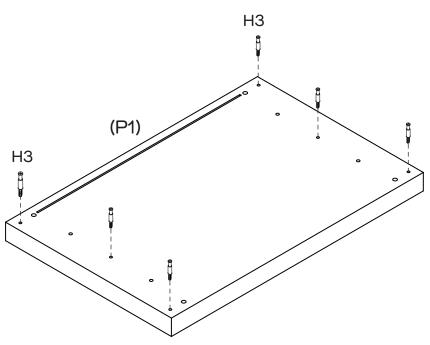
Secure 6 x Cam Bolts (H3) to Top Panel (P1) by tightening with the Phillips Head Screwdriver.
