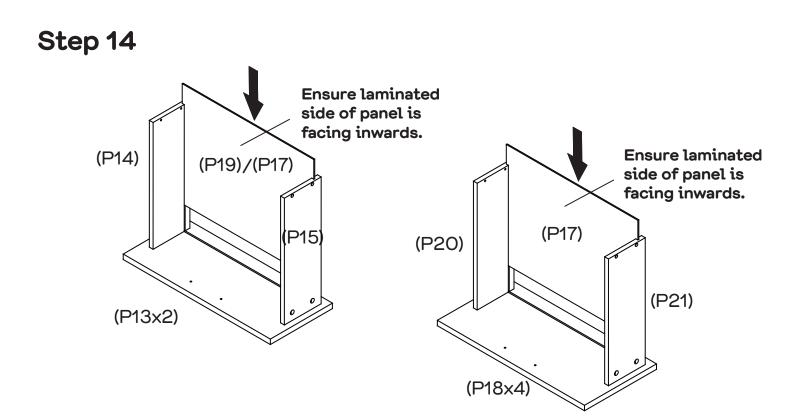
Slide the Drawer Bases (P17x5) into the grooves of Left & Right Drawer Side (P14 & P15, P20x4 & P21x4) as shown. Slide the Drawer Base (P19) into the grooves of Left & Right Drawer Side (P14 & P15) as shown.
