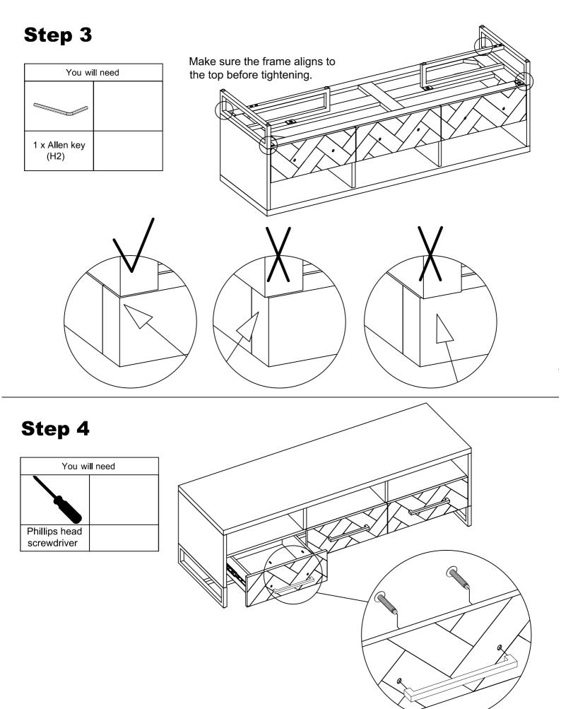
The handles are fitted on the inside of the drawers to protect them during transport. Open the drawers, unscrew the handles, and then fix them on the outside as shown.
