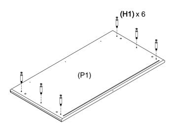
Fix 6 x Cam Bolts (H1) to Top Panel (P1) by using a Phillips head screwdriver.
