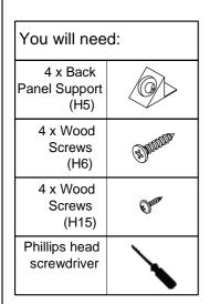
Fix Back Panel (P11) to Back Rail (P9) by using 4 Wood Screws (H15). Fix Back Panel Support (H5) to each corner on the back by using Wood Screws (H6).
