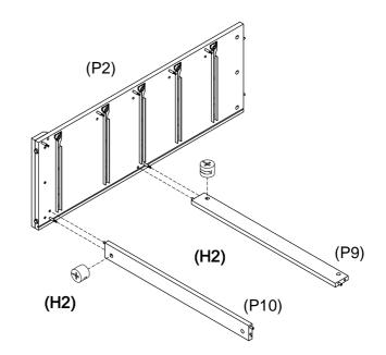
Attach Back Support Rail (P10) and Back Rail (P9) to Left Side (P2), insert Cam Nut (H2) into Rail(P9, P10), rotate the Cam Nuts so the arrow point towards the incoming cam bolt, turn clockwise to lock.
