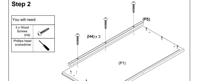
Attach Top Panel Rail (P5) to Top Panel (P1) by using 3 Wood Screws (H4) and a Philip head screwdriver.
