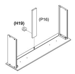
Attach Drawer Support Rail (P16) to Drawer Front (P12), insert small Cam Nut (H19) and use a Philip head screw driver turn clockwise to lock.
