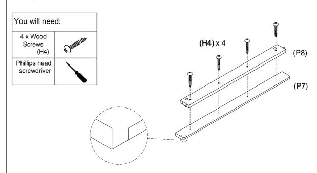
Attach Front Suport Rail (P8) to Front Plinth (P7) by using 3 Wood Screws (H4) and a Philip head screwdriver.
