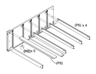
Attach Front Rails (P6) and Front Support Rail (P8) to Left Side (P2), insert Cam Nut (H2) into Rail(P6, P8), rotate the Cam Nuts so the arrow point towards the incoming cam bolt, turn clockwise to lock.
