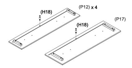
Fix small Cam Bolts (H18) to Drawer Front (P12) and Large Drawer Front (P17) by using a Phillips head screwdriver.
