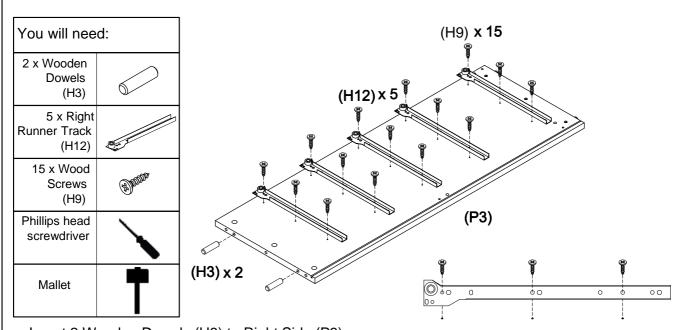
Insert 2 Wooden Dowels (H3) to Right Side (P3). Fix 5 Right Runner Track (H12) to Right Side (P3) by using 15 Wood Screw (H9) and a Phillips head screwdriver.
