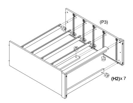
Attach Right Side (P3) to all the Rails which already attached to Left Side (P2), insert Cam Nut (H2) into Rail(P9, P10), rotate the Cam Nuts so the arrow point towards the incoming cam bolt, turn clockwise to lock.
