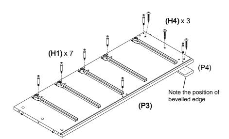
Attach Side Plinth (P4) to Right Side (P3) by using 3 Wood Screws (H4) and a Philip head screwdriver.
