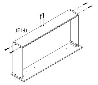
Use Wood Screws (H10) to fix Drawer Back panel to Drawer Sides and Drawer Support Rails.
