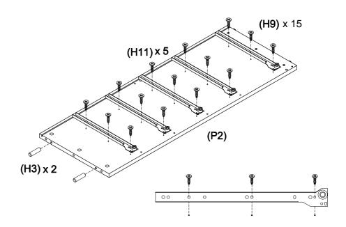
Insert 2 Wooden Dowels (H3) to Left Side (P2). Fix 5 Left Runner Track (H11) to Left Side (P2) by using 15 Wood Screw (H9) and a Phillips head screwdriver.
