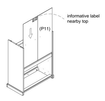
Turn the unit upright carefully, slip Back Panel (P11) into the grooves on the side panels, make sure the infirmative label on position as the drawing shown.
