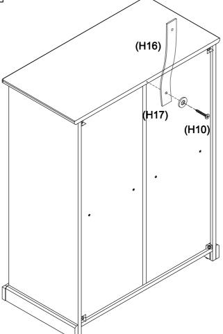
Fix Wall Strap (H16) to back of the Top Panel by using Wood Screw (H10) and Washer (H17).
