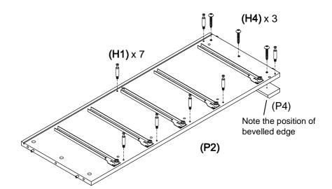
Attach Side Plinth (P4) to Left Side (P2) by using 3 Wood Screws (H4) and a Philip head screwdriver.
