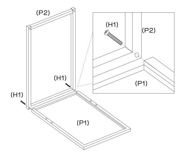
Align the holes on the table top (P1) with the holes on side frame (P2) as shown. Secure together using  $2 \times 1000$  bolts (H1), tightening using allen key (H3).
