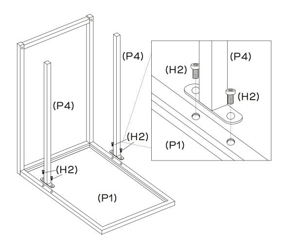
Align the holes on the table top (P1) with the holes on the  $2 \times tubes$  (P4). Attach together using  $4 \times tuber$  (H2), tightening using the allen key (H3).
