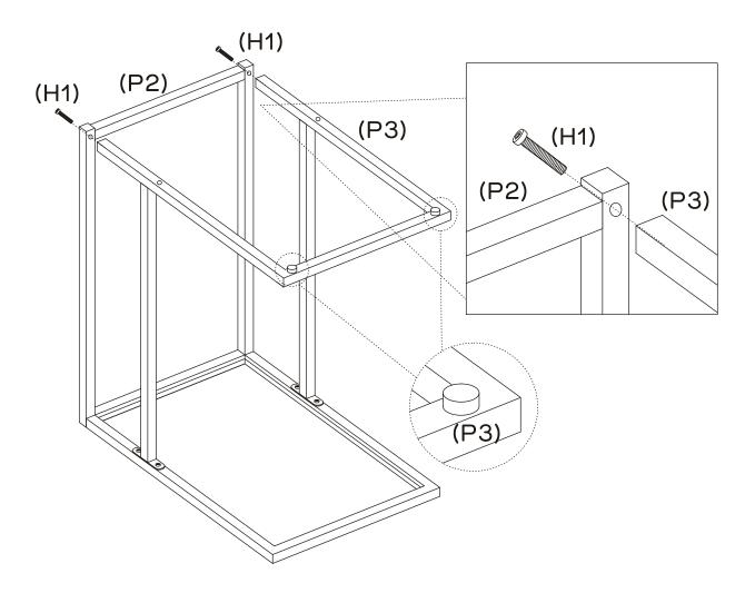
Align the holes on the bottom frame (P3) with the holes on the side frame (P2) as shown. Ensure the holes in the middle of the bottom frame (P3) also align with the 2 x tubes (P4). Secure the side frame (P2) and bottom frame (P3) together using 2 x long bolts (H1), tightening with allen key (H3).
