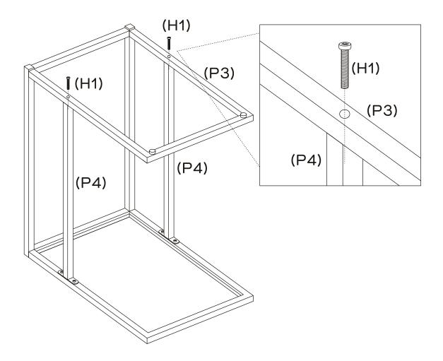
Ensure the holes on the bottom frame (P3) and  $2 \times tubes$  (P4) are aligned. Secure together using  $2 \times long$  bolts (H1), tightening with allen key (H3). Carefully turn the table upright.
