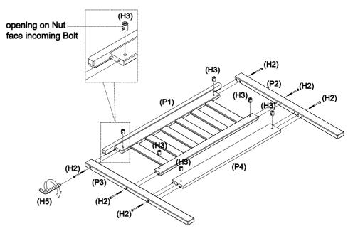
Attach 2 x legs (P2 & P3) to the headboard core (P1) and headboard rail (P4). Insert 6 x nuts (H3) into the headboard rail (P4) and headboard core (P1) as shown. Make sure the opening on the nuts (H3) is facing the incoming bolts, then insert 6 x large bolts (H2), use the allen key (H5) and turn clockwise to fix.
