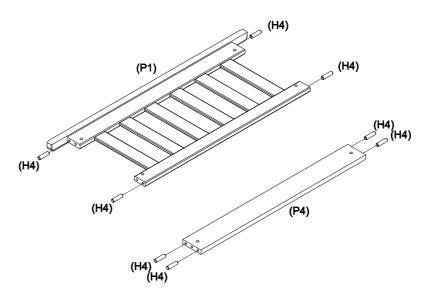
Insert 8 x wooden dowels (H4) into the headboard core (P1) and headboard rail (P4) as shown, using a soft head mallet.
