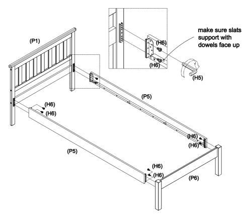
Connect the 2 x side rails (P5) to the headboard (P1) and footboard (P6), using an allen key (H5), turn 8 x small bolts (H6) clockwise to fix.
