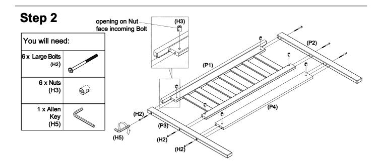
Attach 2 x legs (P2 & P3) to the headboard core (P1) and headboard rail (P4). Insert 6 x nuts (H3) into the headboard rail (P4) and headboard core (P1) as shown. Make sure the opening on the nuts (H3) is facing incoming bolts, then insert 6 x large bolts (H2), use the allen key (H5) and turn clockwise to fix.
