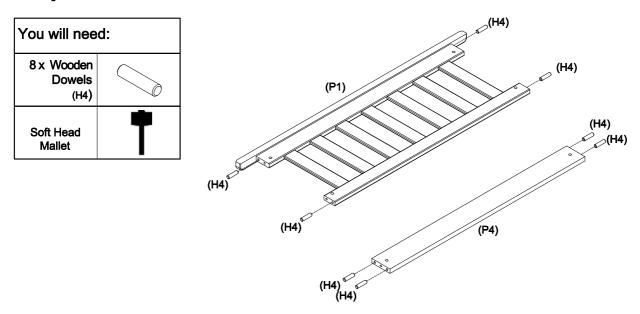
Insert 8 x wooden dowels (H4) into the headboard core (P1) and headboard rail (P4) as shown, using a soft head mallet.
