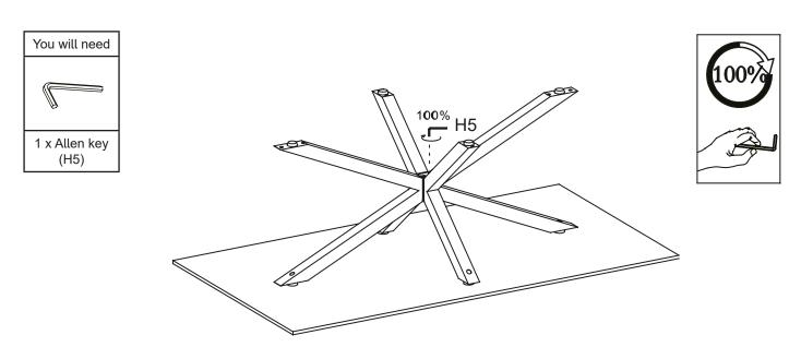
Make sure the table is level, then fully tighten all bolts (H1) by using allen key (H5).
