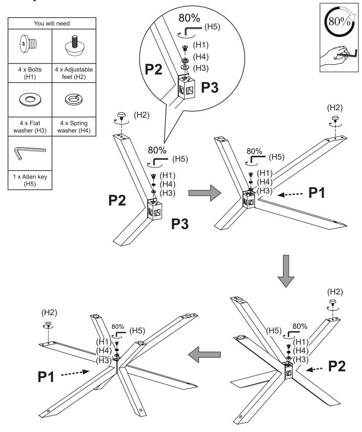
Attach adjustable feet (H2) to legs (P1 and P2).
