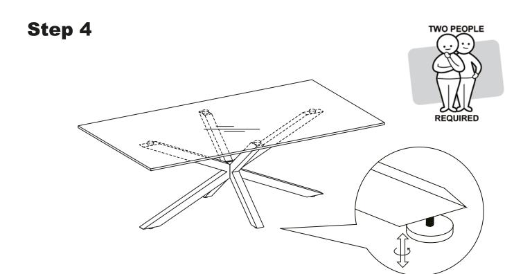
Carefully turn the table to its upright position. Adjust height by adjusting feet.
