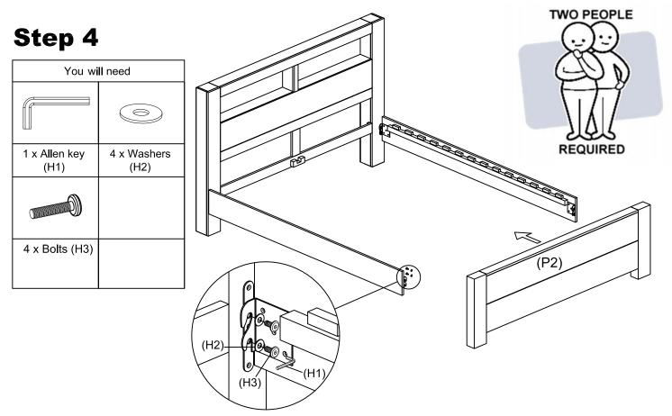
Attach the Footboard (P2) to 2 x Side rails (P3) using 4 x Bolts (H3) and 4 x Washers (H2) as shown. Tighten the Bolts (H3) with Allen key (H1). www.fantasticfurniture.com.au
