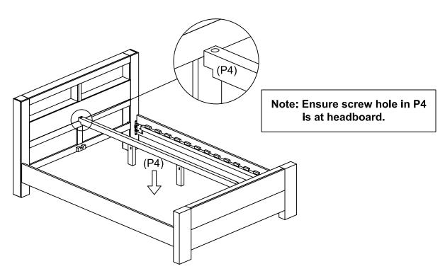
Place the Center rail (P4) into the Bed frame.
