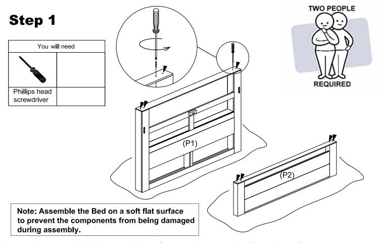
Turn the Headboard (P1), Footboard (P2) upside down (Bottom Up). Using a Screwdriver, loosen the 8 Screws and remove the Plywood brace.
