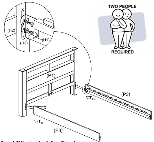
Attach 2 x Side rails (P3) to the Headboard (P1) using 4 x Bolts (H3) and 4 x Washers (H2) as shown. Tighten the Bolts (H3) with Allen key (H1).
