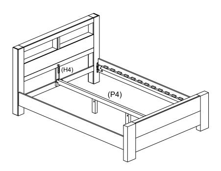
Fix the Center rail (P4) into the Headboard with Screws (H4).
