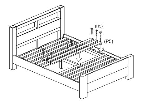
Place the Slats (P5) into the Bed frame, fix the Slats to the Bed frame with Screws (H5).
