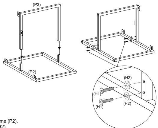
Fix the legs frame (P3) to legs frame (P2). Using 8 bolts (H1) & 8 washers (H2).
