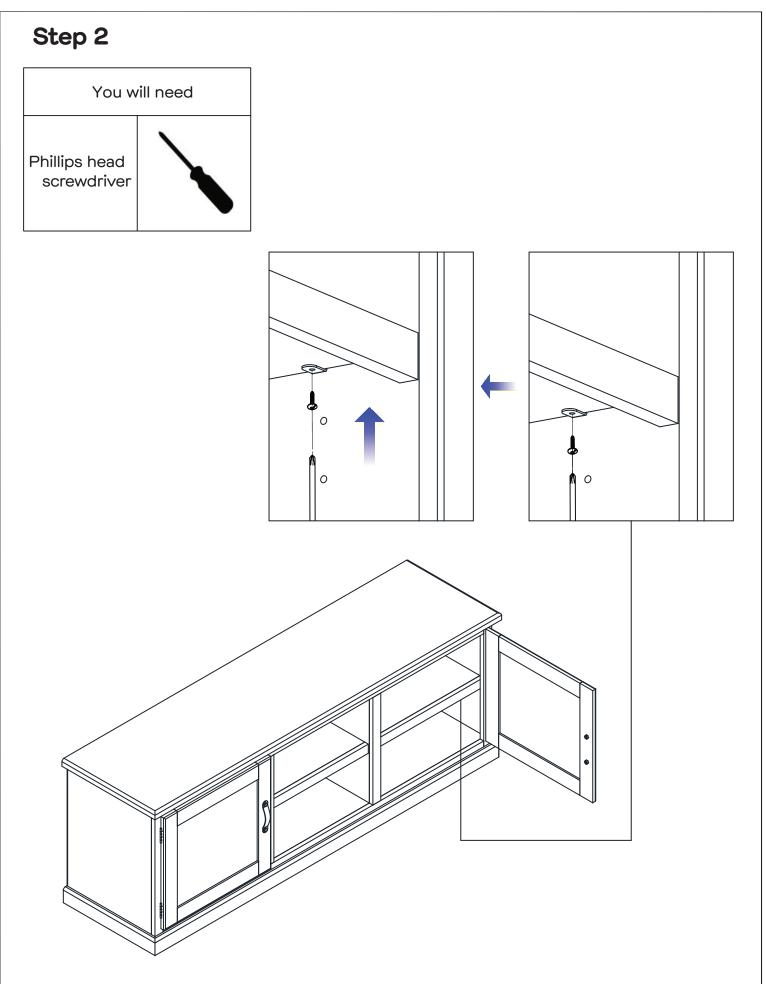
Shelf height is adjustable. Before adjusting any shelf, remove all screws underneath the shelf.
