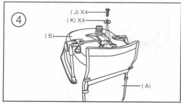
Attach back support (A) into seat plate (D) using screws (J) and flat washers (K). Fully tighten screws.
