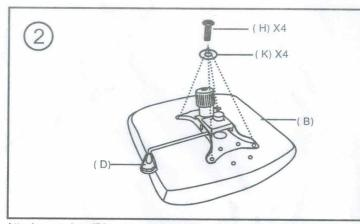
Attach seat plate (D) to seat cushion (B), using screws (H) and flat washers (K). Fully tighten screws.
