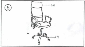
With base (F) upright and castors (G) on the floor, insert pneumatic cylinder (E) into base (F). Place the assembled seat on top of pneumatic cylinder (E) and apply downward pressure.
