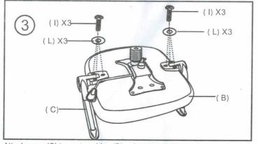
Attach arms (C) to seat cushion (B) using screws (I) and flat washers (L). Fully tighten screws.
