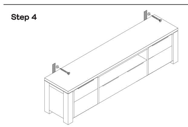
Unwrap lowline large and move into final position. Seek advice from a qualified trades person on how to attach the safety strap to your specific wall.
