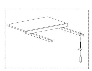
Remove the six transport locking screws.
