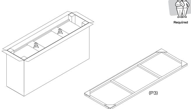
Turn the carton upside down (Bottom up). Open the carton and remove the pallet (P3).
