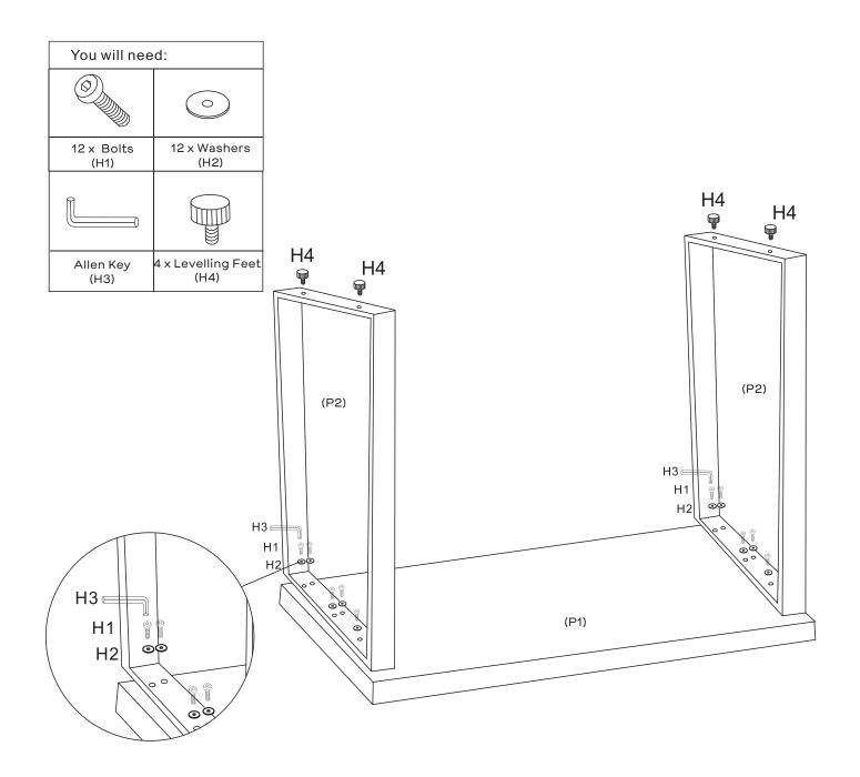
Secure 2 x Legs (P2) to Desk Top (P1) with 12 x Washers (H2) and by tightening  $12 \times Bolts$  (H1) with the Allen Key (H3) as shown. Attach  $4 \times Levelling$  Feet (H4) to the bottom of Legs (P2x2) by gently screwing in. If the floor is uneven, the Levelling Feet can be adjusted as needed.
