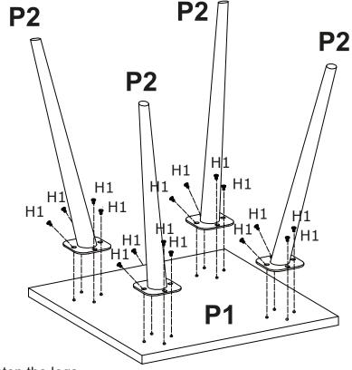
Place legs (P2) on the table top (P1). Use bolts (H1) and allen key (H2) to fasten the legs.
