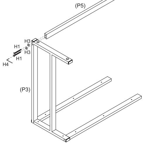
Attach Rail (P5) to Right Frame (P3) with 2 x Long Bolts (H1) and 2 x Washers (H3). Tighten the bolts using an Allen Key (H4).
