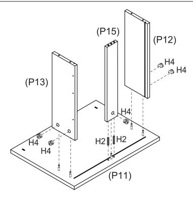
Insert 2 x Small Dowels (H2) into the holes of Drawer Front (P11) as shown.
