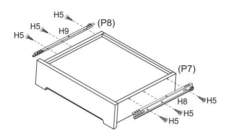
Attach 1 x DL Runner (H8) to Left Drawer Side (P7) and 1 x DR Runner (H9) to Right Drawer Side (P8) with 6 x Small Screws (H5). Repeat Step 8 to Step 12 to assemble another drawer.
