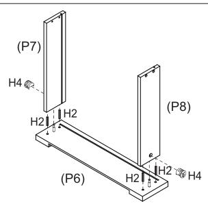
Insert 4 x Small Dowels (H2) into the holes of Drawer Front (P6) as shown. Insert 2 x Cam Nuts (H4) into the holes of Drawer Sides (P7, P8).
