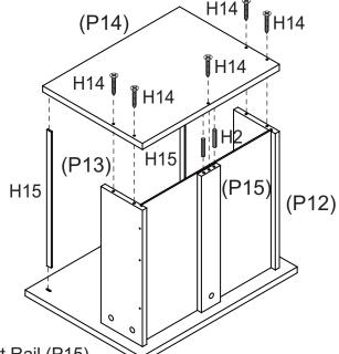
Insert 2 x Small Dowels (H2) into Support Rail (P15).
