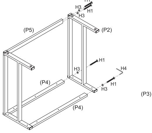
Attach Left Frame (P2) to Rails (P4, P5) with 4 x Long Bolts (H1) and 4 x Washers (H3). Tighten the bolts using an Allen Key (H4).
