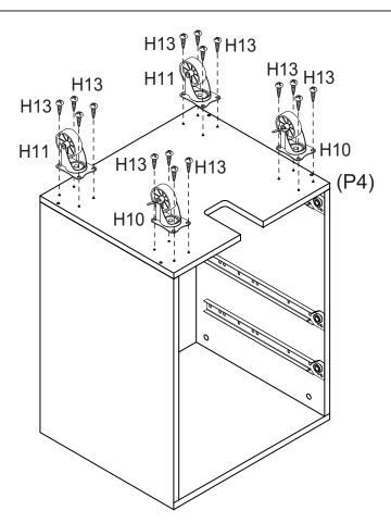
Attach 2 x Front Wheels (H10) and 2 x Wheels (H11) to Bottom Panel (P4) with 16 x Round Screws (H13) using a Phillips head screwdriver.
