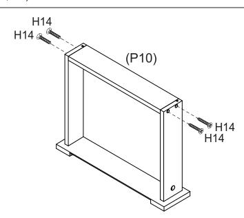
Attach Drawer Back (P10) to Drawer Sides (P7, P8) with 4 x Long Screws (H14), make sure that the groove lines up the whole way around the drawer. Tighten Screws using a Phillips head screwdriver.
