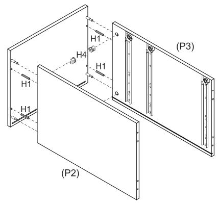
Insert 4 x Dowels (H1) into Side Panels (P2, P3).
