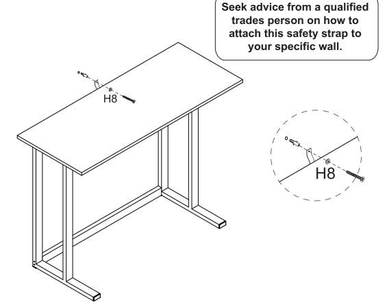
Move the desk to the final position, and attach the safety strap to the wall securely. Make sure it is firmly attached and snug fit.
