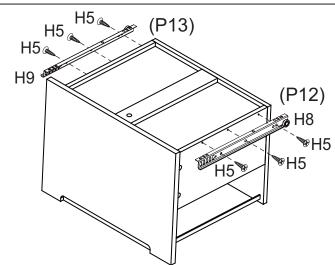
Attach 1 x DL Runner (H8) to Left Drawer Side (P12) and 1 x DR Runner (H9) to Right Drawer Side (P13) with 6 x Small Screws (H5).
