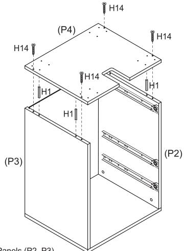
Insert 4 x Dowels (H1) into Side Panels (P2, P3).
