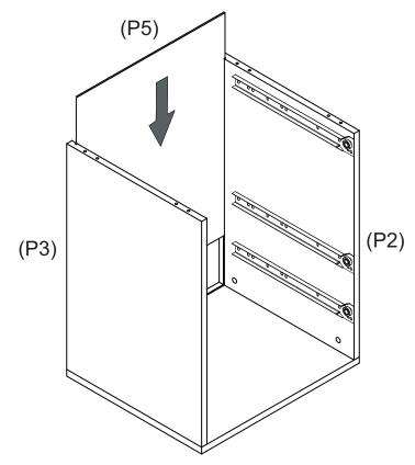
Carefully turn the frame over to an upright position. Slide Back Panel (P5) in through the grooves of Side Panels (P2, P3) as shown.
