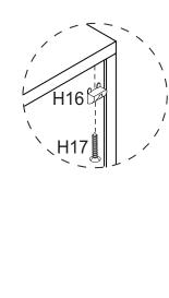
Secure Back Panel (P5) in place with 4 x Wedges (H16) using 4 x Screws (H17). Tighten Screws using a Phillips head screwdriver.
