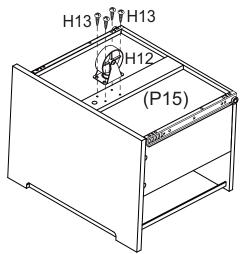
Attach 1 x Large Wheel (H12) to Support Rail (P15) with 4 x Round Screws (H13) using a Phillips head screwdriver.
