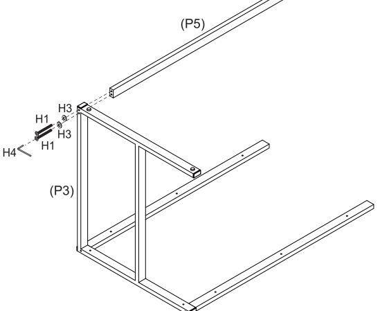
Attach Rail (P5) to Right Frame (P3) with 2 x Long Bolts (H1) and 2 x Washers (H3). Tighten the bolts using an Allen Key (H4).
