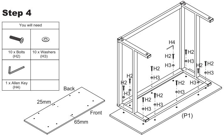
Put Top Panel (P1) on a soft flat surface as shown. Attach the frame to Top Panel (P1) with 10 x Bolts (H2) and 10 x Washers (H3) using an Allen Key (H4). Check and tighten all bolts.
