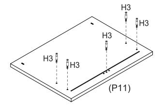
Insert 5 x Cam Bolts (H3) into Drawer Front (P11) with a Phillips head screwdriver.
