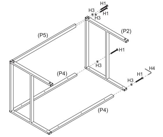
Attach Left Frame (P2) to Rails (P4, P5) with 4 x Long Bolts (H1) and 4 x Washers (H3). Tighten the bolts using an Allen Key (H4).
