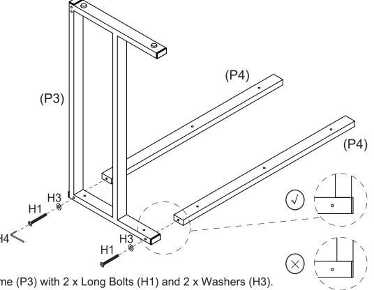
Attach Rails (P4) to Right Frame (P3) with 2 x Long Bolts (H1) and 2 x Washers (H3). Tighten the bolts using an Allen Key (H4).
