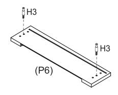
Insert 2 x Cam Bolts (H3) into Drawer Front (P6) with a Phillips head screwdriver.
