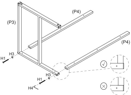
Attach Rails (P4) to Right Frame (P3) with 2 x Long Bolts (H1) and 2 x Washers (H3).
