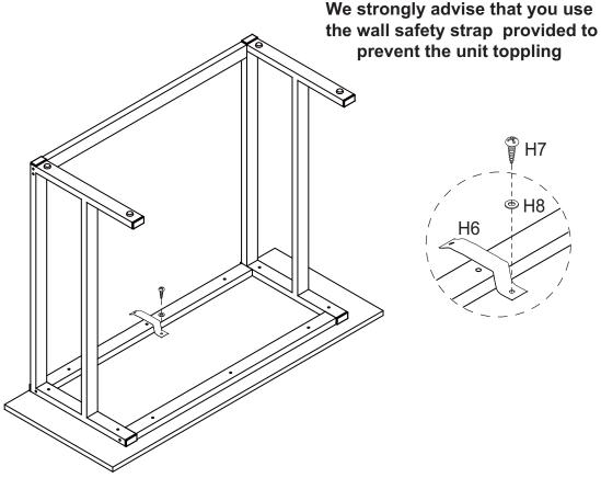
Use Screw (H7) and Washer (H8) to attach Safety Strap (H6) securely on the bottom of Top Panel (P1) as shown.
