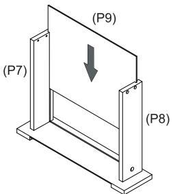
Slide Drawer Base (P9) into the grooves of Drawer Sides (P7, P8).
