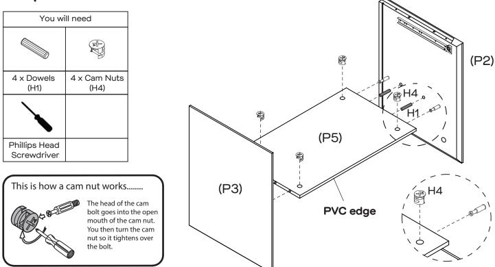
Attach Left Side Panel (P2) and Right Side Panel (P3) to Shelf Panel (P5) with  $4 \times 1$  Dowels (H1) and secure with  $4 \times 1$  Cam Nuts (H4). Tighten with a Phillips Head Screwdriver.
