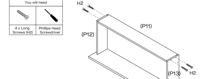
Attach Drawer Back (P11) to Drawer Sides (P12, P13) with  $4 \times 1$  Long Screws (H2), make sure that the groove lines up the whole way around the drawer. Tighten with a Phillips Head Screwdriver.
