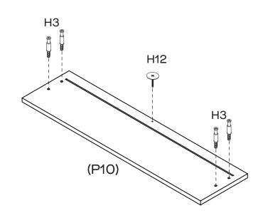
Attach  $4 \times \text{Cam}$  Bolts (H3) and  $1 \times \text{Screw}$  (H12) to Drawer Front (P10) as shown. Tighten with a Phillips Head Screwdriver.
