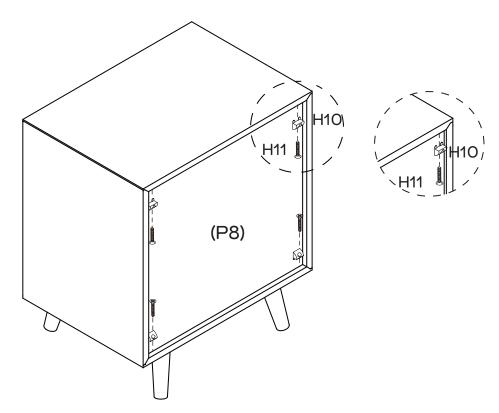
Secure Back Panel (P8) in place with 4 x Wedges (H10) using 4 x Wedge Screws (H11). Tighten with a Phillips Head Screwdriver.
