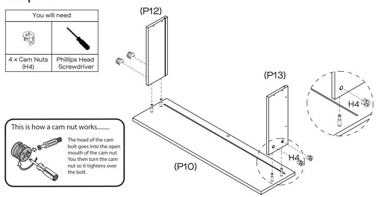
Attach Drawer Sides (P12, P13) to Drawer Fronts (P10). Insert 4 x Cam Nuts (H4) into the holes of Drawer Sides (P12, P13). Make sure the opening on cam nuts point towards the incoming cam bolts. Tighten with a Phillips head screwdriver.
