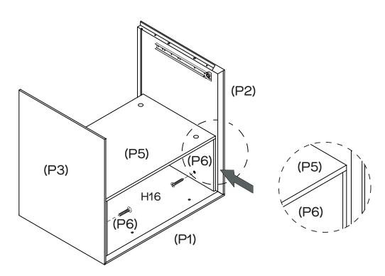
Press 2 x Shelf Panels (P6) against Shelf Panels (P2,P3), then slide 2 x Shelf Panels (P6) between Shelf Panels (P5) and Top Panel (P1) to form the unit as shown. Attach 2 x Shelf Panels (P6) to Left Side Panel (P2) and Right Side Panel (P3) secure with 4 x Screws (H16). Tighten with a Phillips Head Screwdriver.
