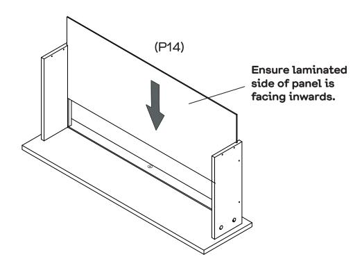
Slide the Drawer Base (P14) into the grooves between drawer sides as shown.
