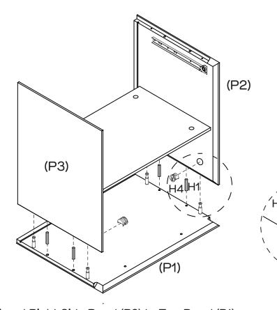
Attach Left Side Panel (P2) and Right Side Panel (P3) to Top Panel (P1) with 4 x Dowels (H1) and secure with 4 x Cam Nuts (H4). Tighten with a Phillips Head Screwdriver.
