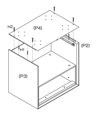
Attach Bottom Panel (P4) to Left Side Panel (P2) and Right Side Panel (P3) with 4 x Dowels (H1) and secure with 4 x Long Screws (H2). Tighten with a Phillips Head Screwdriver.
