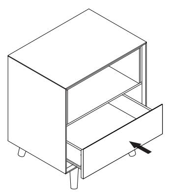
To open the drawer, firmly press the middle of the drawer front to trigger the Catch to bounce the drawer open. If the drawer does not pop open when pressed or is not sitting flush with the front of the unit, reach to the Rail and adjust the head of the Catch by gently turning left or right to reach the right resistance.
