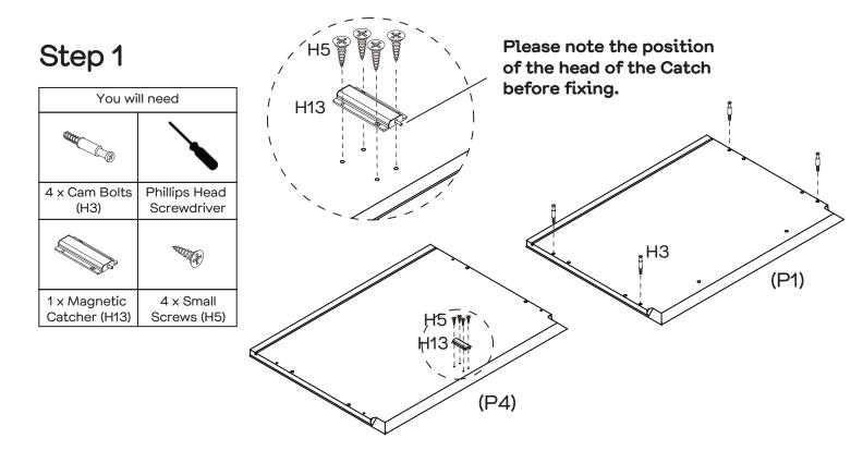
Attach 4 x Cam Bolts (H3) to Top Panel (P1) as shown. Tighten with using a Phillips Head Screwdriver. Attach 1 x Magnetic Catcher (H13) to Bottom Panel (P4) and secure with 4 x Small Screws (H5). Tighten with a Phillips Head Screwdriver.
