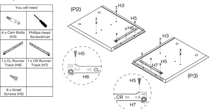
Attach 4 x Cam Bolts (H3) to Left Side Panel (P2) and Right Side Panel (P3) as shown. Tighten with a Phillips Head Screwdriver. Attach  $1 \times CL$  Runner Track (H6) to Left Side Panel (P2) with  $3 \times Small$  Screws (H5). Attach  $1 \times CR$  Runner Track (H7) to Right Side panel (P3) with  $3 \times Small$  Screws (H5). Tighten with a Phillips Head Screwdriver.
