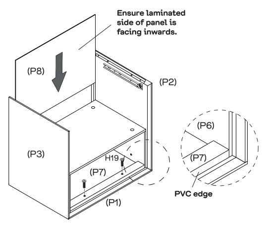
Slide remaining Back Panels (P8) into the groovesof Left Side Panel (P2) and Right Side Panel (P3). Press Rail (P7) against Top Panel (P1), then slide Rail (P7) between Left Side Panel (P2) and Right Side Panel (P3) to form the unit as shown. Attach Rail (P7) to Top Panel (P1) secure with 2 x Small Bolts (H19). Tighten with a Phillips Head Screwdriver.
