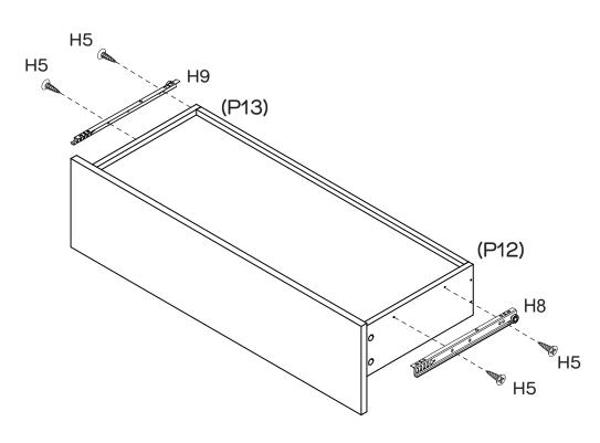
Attach 1  $\times$  DL Runner (H8) to Left Drawer Side (P12) and 1  $\times$  DR Runner (H9) to Right Drawer Side (P13) with 4  $\times$  Small Screws (H5) using a Phillips Head Screwdriver.
