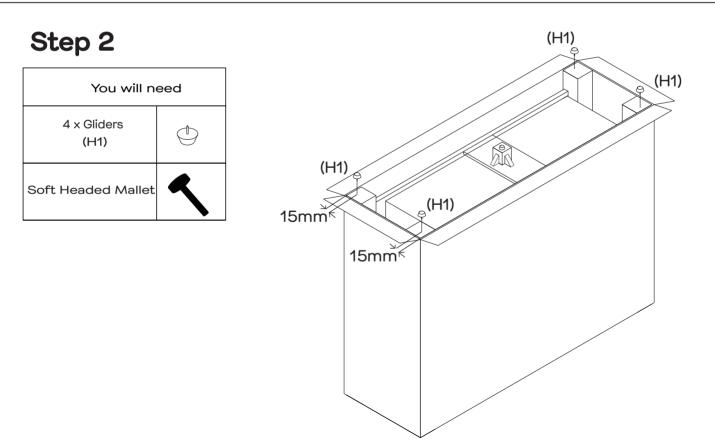
Use a Soft Headed Mallet to nail the gliders (H1) into the middle of the each leg. and approximately 15mm from the front and the back side.
