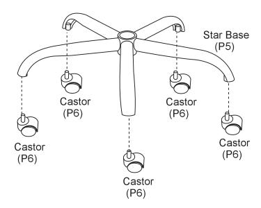
Insert 5 x castors into the star base (P5) one at a time as shown. Push down firmly on each castor to ensure they are fixed into position.
