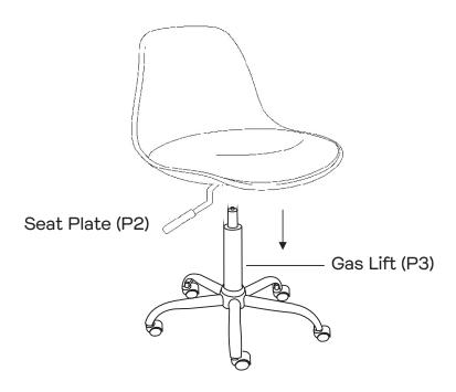
Position the centre on the seat plate (P2) over the top of the gas lift (P3). Carefully lower the seat (P1) onto the gas lift (P3). Carefully and firmly press the seat down firmly to lock it into position. Check the connection is secure before sitting in the chair.
