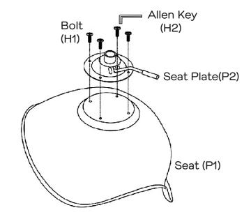
Align the holes of the seat plate (P2) to the holes of the underside of the seat (P1). Attach the seat plate (P2) to the underside of the seat (P1) with 4xbolts(H1) using an allen key (H2).
