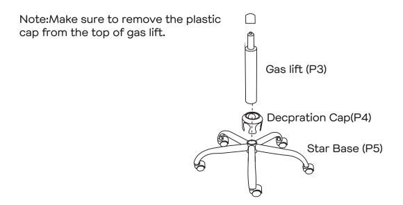
Remove the plastic cap from the top of the gas lift (P3). Place the decoration cap (P4) over the top of the star base (P5). Insert the gas lift (P3)through the decoration cap (P4) and into the star base (P5) as shown.
