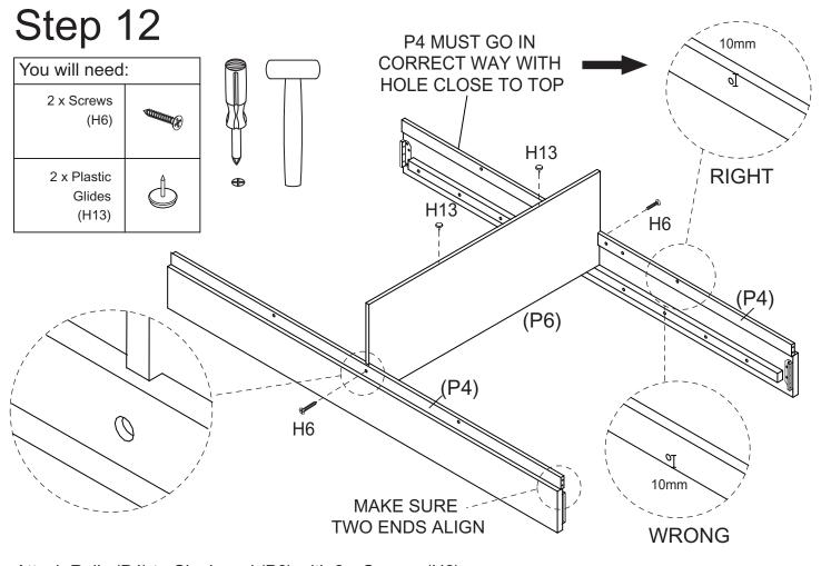
Attach Rails (P4) to Clapboard (P6) with 2 x Screws (H6). Then hammer 2 x Plastic Glides (H13) on the bottom of Clapboard (P6).
