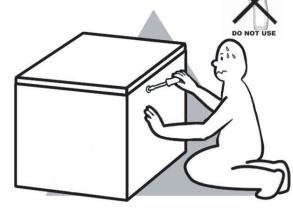
**DO NOT** fully tighten screws (leave slightly loose). When the item is fully assembled tighten the screws - but do not over tighten.
