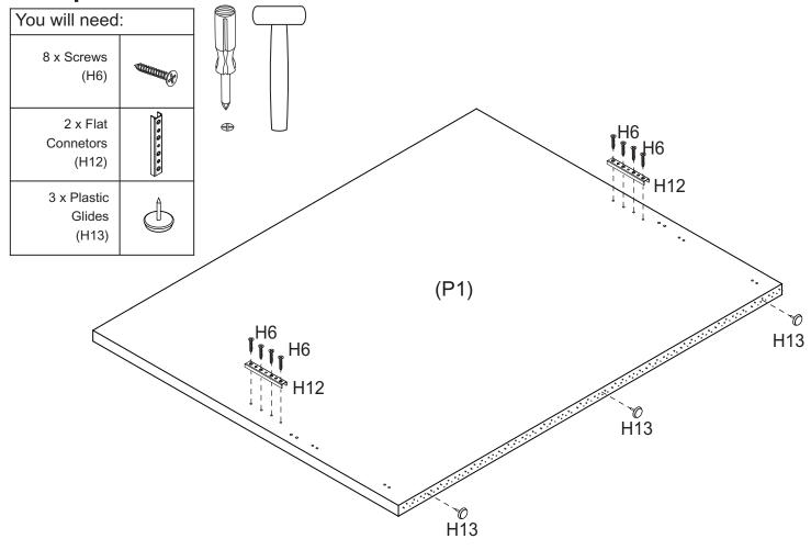
Attach 2 x Flat Connectors (H12) to Bedhead (P1) with 8 x Screws (H6). Then hammer 3 x Plastic Glides (H13) on the bottom of Bedhead (P1).
