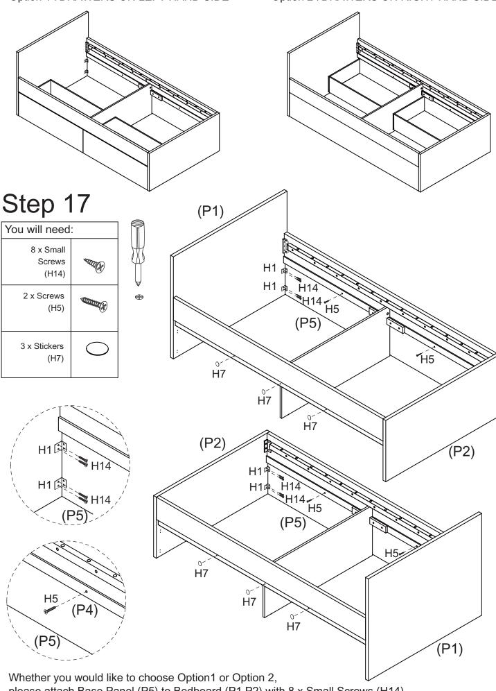
please attach Base Panel (P5) to Bedboard (P1,P2) with 8 x Small Screws (H14). Attach Base Panel (P5) to Rails (P4) with 2 x Screws (H5). Attach 3 x Stickers (H7) to the holes of Rail (P4).
