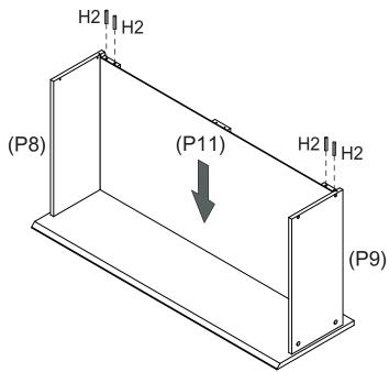
Slide Drawer Base (P11) into the groove in the Drawer Sides (P8,P9). Insert 4 x Small Dowels (H2) into Drawer Support (P13).
