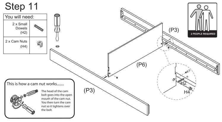
Insert 2 x Small Dowels (H2) into Side Rails (P3).
