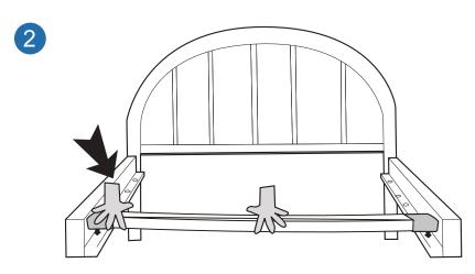
Place the slat in position then push down in the centre to flatten. Make sure the plastic prong lines up with the hole, then push in firmly.
