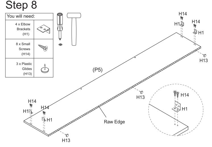
Attach 4 x Elbow Brackets (H1) to Base Panel (P5) with 8 x Small Screws (H14). Then hammer 3 x Plastic Glides (H13) on the bottom of Base Panel (P5).
