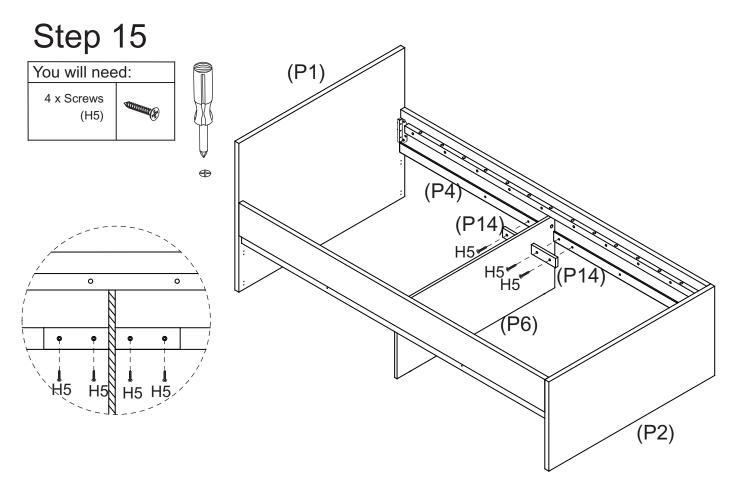
Attach 2 x Blocks (P14) to Rail (P4) with 4 x Screws (H5).
