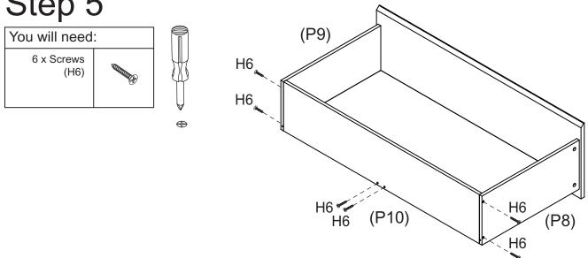
Attach Drawer Back (P10) to Drawer Sides (P8,P9) with 4 x Screws (H6), and Central Drawer Support (P12) with 2 x Screws (H6). Make sure that the groove lines up the whole way around the drawer.
