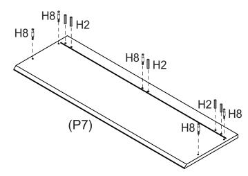
Insert 5 x Small Dowels (H2) into Drawer Front (P7), and attach 5 x Small Cam Bolts (H8) to it.
