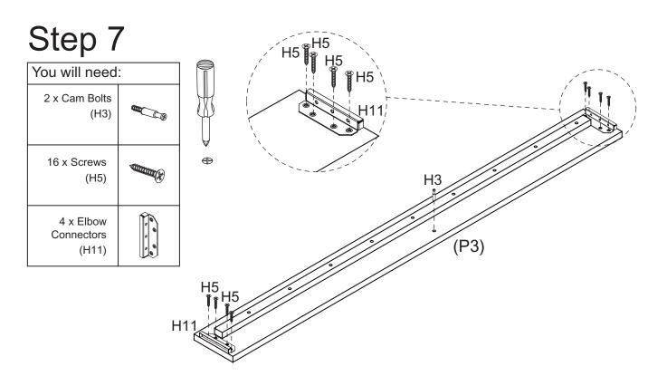
Attach 1 x Cam Bolt (H3) to Side Rail (P3). Attach 2 x Elbow Connectors (H11) to Side Rail (P3) with 8 x Screws (H5). Repeat Step 7 again with the other Side Rail (P3).
