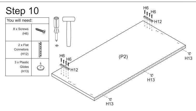
Attach 2 x Flat Connectors (H12) to Bedfoot (P2) with 8 x Screws (H6). Then hammer 3 x Plastic Glides (H13) on the bottom of Bedfoot (P2).
