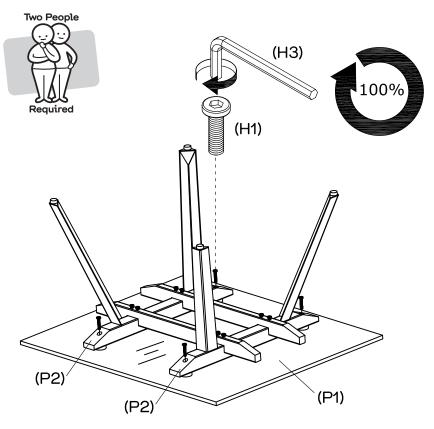
Lay table top (P1) onto a soft flat surface to avoid damaging the glass. With assistance, lay the assembled leg frame (P2,P3) onto table top (P1) and align the holes. Attach the legs (P2) to table top (P1) using 4 x small bolts (H1). Do not fully tighten the bolts (H1) until they have all been inserted into the holes. Once they have been inserted, you may fully tighten the bolts.
