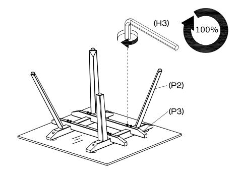
You may now fully tighten the  $8 \times 1$  large bolts attaching the legs (P2) to rails (P3) using allen key (H3).
