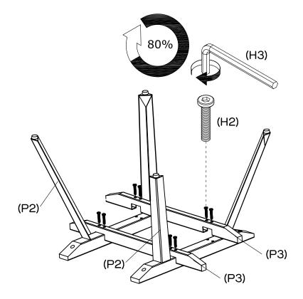
Attach 2 x rails (P3) to 2 x legs (P2), by using 8 x large bolts (H2) and allen key (H3). Do not fully tighten bolts, tighten only to 80 %.
