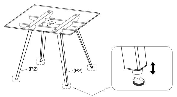
With assistance, carefully turn over the lamp table so it is upright. If required, you can extend the foot on each leg by turning it anti-clockwise, or clockwise as required, to ensure the table is level with the ground.
