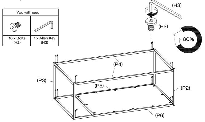
Secure the Top Rails and Middle Rail (P5,P6&P7) and the Bottom Rails (P4x2) to the End Frame Left & Right (P2&P3) with 16 x Bolts (H2) by tightening with the Allen Key (H3). Do not fully tighten Bolts, tighten only to 80 %
