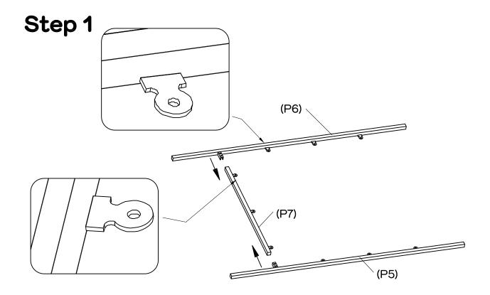
Attach the Top Rails (P5&P6) to the Middle Rail (P7) as shown. Ensure the metal tabs on the Top Rails (P5&P6) and Middle Rail (P7) are rotated into shown position.
