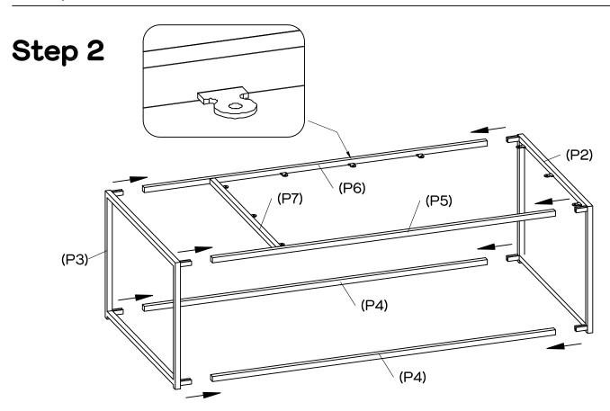
Attach the assembled Top and Middle Rails (P5,P6&P7) and the Bottom Rails (P4x2) to the End Frame Left & Right (P2&P3) as shown.
