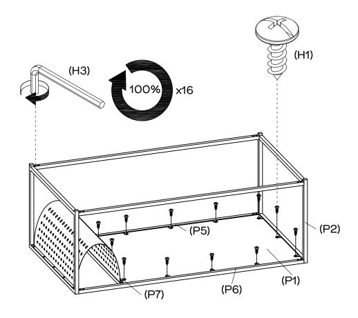
Place the Top (P1) into the assembled frame as shown.
