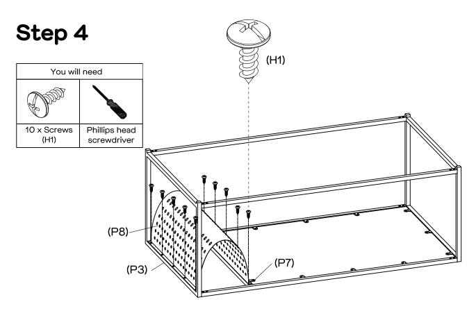
Attach the Rack Base (P8) to the End Frame Left (P3) and Middle Rail (P7) using Screws (H1) and Phillips Head Screwdriver
