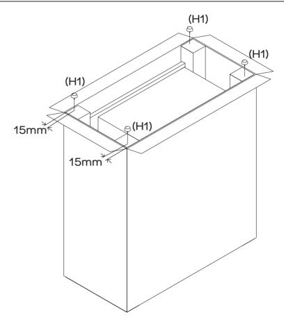
Use a Soft Headed Mallet to nail the gliders (H1) at the middle of the legs and approximately 15mm from the front and the back side.
