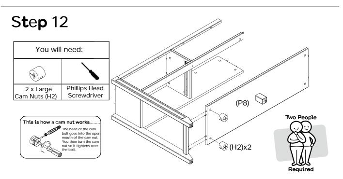
With assistance, attach bottom shelf (P8) to left side (P2). Insert 2 x large cam nuts (H2) into the bottom shelf (P8). Using a phillips head screwdriver, rotate the cam nut so the arrow points towards the incoming cam bolts. Turn clockwise to lock.
