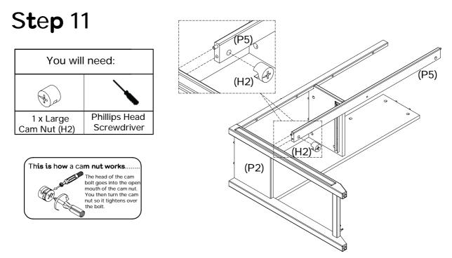
Attach front support rail (P5) to left side, ensuring the side with cam nut holes faces down. Insert 1 x large cam nut (H2) into support rail (P5). Using a phillips head screwdriver, rotate the cam nut so the arrow points towards the incoming cam bolt. Turn clockwise to lock.
