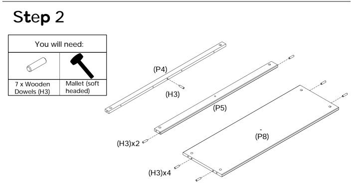
Insert 7 x wooden dowels (H3) into top panel rail (P4), front support rail (P5) and bottom shelf (P8) as shown.
