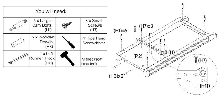
Attach 6 x large cam bolts (H1) to left side (P2) using a phillips head screwdriver. Insert 2 x wooden dowels (H3) into left side (P2).
