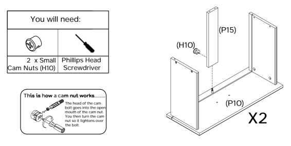
Attach 1 x drawer support rail (P15) to drawer front (P10), ensuring the side with the cam nut hole faces outwards. Insert 1 x small cam nut (H10) into drawer support rail (P15). Using a phillips head screwdriver, rotate the cam nut so the arrow points towards incoming cam bolt. Turn clockwise to lock.
