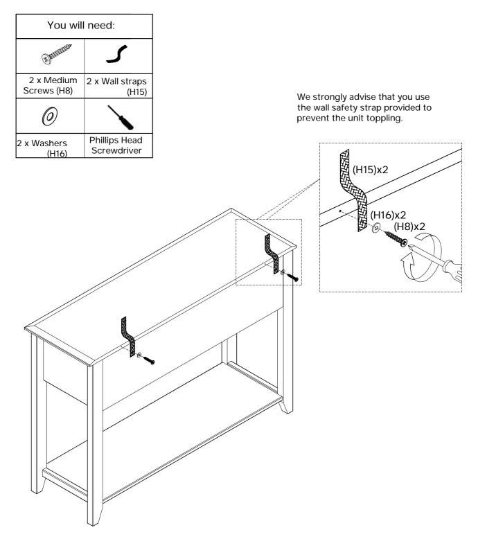
Attach 2 x wall straps (H15) to the back of the top panel (P1) using 2 x medium screws (H8) and 2 x washers (H16), tightening using a phillips head screwdriver.
