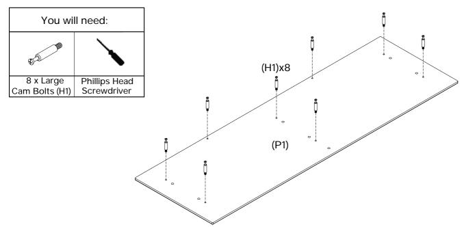
Attach 8 x large cam bolts (H1) to top panel (P1) using a phillips head screwdriver.
