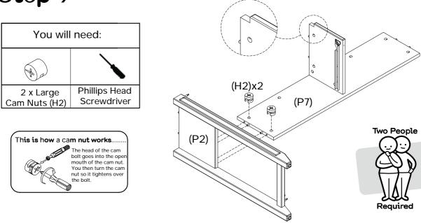
With assistance, attach back panel (P7) to left side (P2). Insert 2 x large cam nuts (H2) into back panel (P7). Using a phillips head screwdriver, rotate the cam nuts so the arrow points towards the incoming cam bolt. Turn clockwise to lock.
