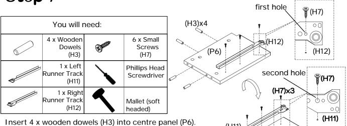
Insert 4 x wooden dowels (H3) into centre panel (P6). Attach 1 x right runner track (H12) to the left side of the centre panel (P6) using 3 x small screws (H7), tightening with a phillips head screwdriver.
