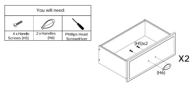
Attach 1 x handle (H6) to assembled drawer using 2 x handle screws (H5), tightening using a phillips head screwdriver. Repeat this process for the other handle (H6).
