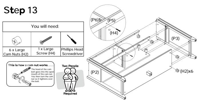
With assistance, attach right side (P3) to the assembled unit. Insert 6 x large cam nuts (H2) into the top panel rail (P4), front support rail (P5) and bottom shelf (P8). Using a phillips head screwdriver, rotate the cam nuts so the arrow points towards the incoming cam bolts. Turn clockwise to lock.
