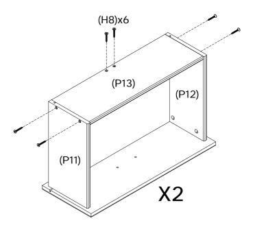
Attach 1 x drawer back panel (P13) to drawer sides (P11, P12) and drawer support rail (P15) using 6 x medium screws(H8), tightening with a phillips head screwdriver. Repeat this process for the other drawer back panel (P13).
