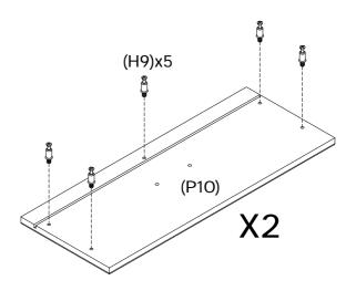
Attach 5 x small cam bolts (H9) to drawer front (P10) using a phillips head screwdriver. Repeat this process for the other drawer front.
