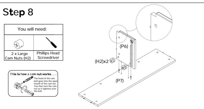
Attach centre panel (P6) to back panel (P7). Insert 2 x large cam nuts (H2) into the centre panel (P6). Using a phillips head screwdriver, rotate the cam nuts so the arrow points towards the incoming cam bolt. Turn clockwise to lock.
