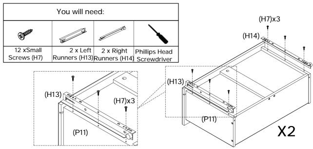
Attach 1 x left runner (H13) and 1 x right runner (H14) to the bottom of drawer sides (P11, P12), ensuring the stoppers are at the back of the assembled drawer, using 6 x small screws (H7) and tightening with a phillips head screwdriver. Repeat this process for the other set of runners (H13, H14).
