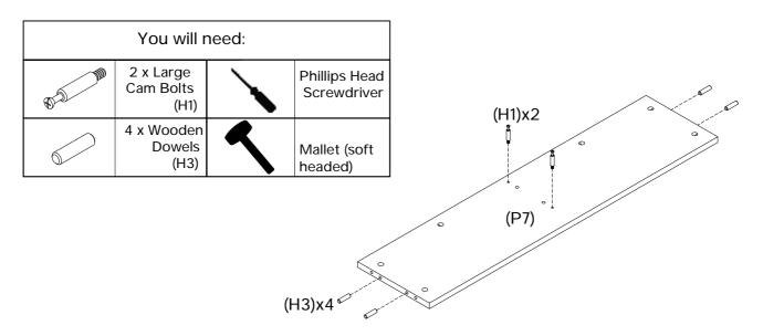
Attach 2 x large cam bolts (H1) to back panel (P7) using a phillips head screwdriver. Insert 4 x wooden dowels (H3) into back panel.
