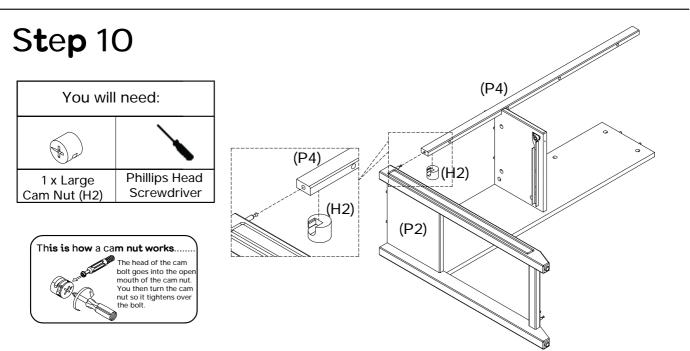
Attach top panel rail (P4) to left side (P2), ensuring the side with cam nut holes faces inwards. Insert 1 x large cam nut (H2) into top panel rail (P4). Using a phillips head screwdriver, rotate the cam nuts so the arrow points towards the incoming cam bolt. Turn clockwise to lock.
