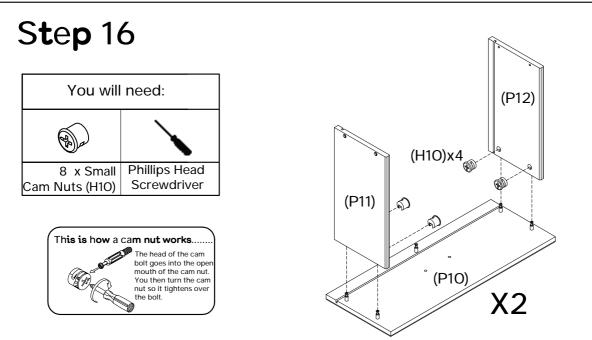
Attach 1 x left drawer side (P11) and 1 x right drawer side (P12) to drawer front, ensuring the grooves on all panels align. Insert 4 x small cam nuts (H10) into drawer sides (P11, P12). Using a phillips head screwdriver, rotate the cam nuts so the arrow points towards incoming cam bolt. Turn clockwise to lock. Repeat this process for the other drawer sides (P11, P12).
