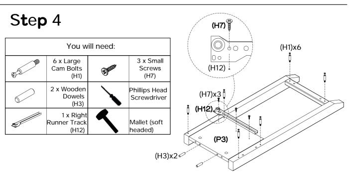
Attach 6 x large cam bolts (H1) to right side (P3) using a phillips head screwdriver. Insert 2 x wooden dowels (H3) into right side (P3).
