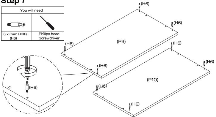
Attach 8 x Cam Bolts (H6) to Drawer Top Panel (P9) and Base Panel (P10) as shown by tightening with the Phillips Head Screwdriver.
