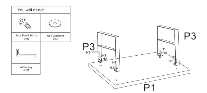
Using 6 x Washers(H2) and 6 x Short Bolts (H1) secure the Table Leg (P3) to the Table Top(P1) by tightening 70% with Allen Key (H3) Repeat step to attach the second Table Leg(P3).
