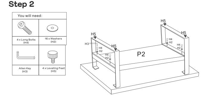
Using 4 x Washers (H2) and 4 x Long Bolts (H4) to secure the Table leg (P3) to the Table Shelf (P2) by tightening with Allen Key (H3) Also tighten the Short Bolts(H1). Screw in 4 x Levelling Feet (H5) to the bottom of Table Legs (P3) Ensure the Levelling Feet are screwed in firmly. If your flooring surface is uneven adjust the Levelling Feet accordingly.
