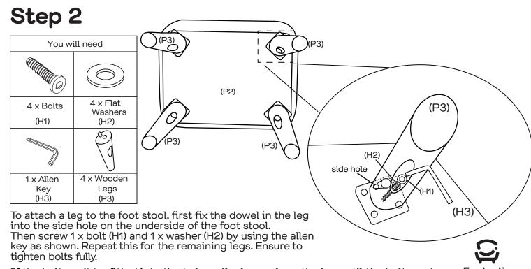
If the bolt can't be fitted into the hole well, please slope the leg until the bolt can be inserted into the hole completely as shown, then screw the bolt to the bottom.
