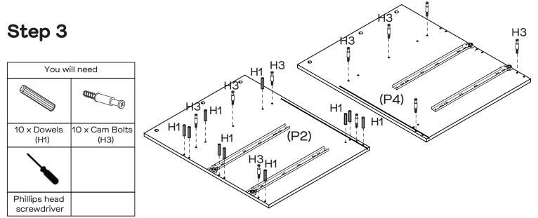
Insert 10 x Dowels (H1) into Left Side Panel (P2). Attach 10 x Cam Bolts (H3) into Left Side Panel (P2) and Divider (P4) by tightening with the Phillips Head Screwdriver as shown
