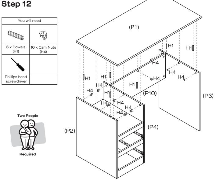
Insert 3 x Cam Nuts (H4) into Left Side Panel (P2), 3 x Cam Nuts (H4) into Divider Panel (P4), 3 x Cam Nuts (H4) into Right Side Panel (P3) and 1 x Cam Nut (H4) into Back Panel (P10). Rotate the cam nuts so the arrows point towards the incoming cam bolts. Insert 2 x Dowels (H1) into Left Side Panel (P2), 2 x Dowels (H1) into Divider Panel (P4) and 2 x Dowels (H1) into Right Side Panel (P3). Attach Top Panel (P1) to the assembled unit by tightening cam nuts with the Phillips Head Screwdriver.
