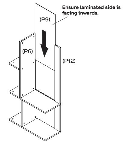
Slide Back panel (P9) into the grooves of the Shelf panel (P6) and Rail (P12) as shown.
