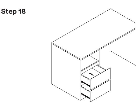
Carefully insert the drawers into the desk by gently guiding the runners into the tracks
