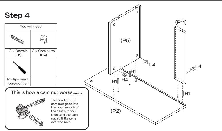
Insert 3 x Dowels (H1) & 3 x Cam Nuts (H4) into Shelf panel (P5) and Rail (P11). Attach Left panel (P2) to Shelf panel (P5) and Rail (P11), secure by tightening Cam Nuts (H4) with a Phillips Head Screwdriver.
