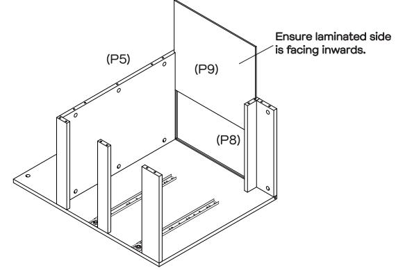
Slide Back Panel (P9) into the groove of Shelf Panel (P5) and Rail (P8).
