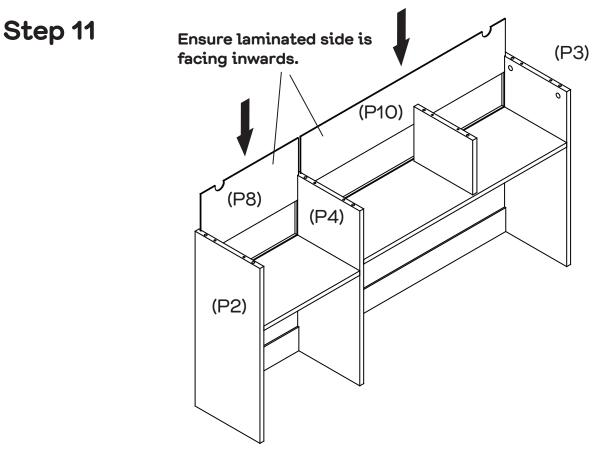
Slide Back panels (P8) & (P10) into the grooves of the Left panel (P2), Divider panel (P4) & Right panel (P3) as shown.
