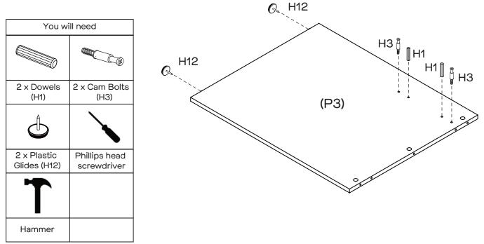
Insert 2 x Dowels (H1) into Right Side Panel (P3). Attach 2 x Cam Bolts (H3) to Right Side Panel (P3) by tightening with the Phillips Head Screwdriver. Use the Hammer to secure the 2 x Plastic Glides (H12) to the bottom of Right Side Panel (P2) as shown.
