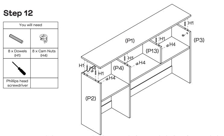
Insert 8 x Dowels (H1) & 8 x Cam Nuts (H4) into the Left Side Panel (P2), Right Side panel (P3), Divider Panel (P4) and Divider Panel (P13). Attach Top Panel (P1) to the unit and secure by tightenir the Cam Nuts (H4) with the Phillips Head Screwdriver.
