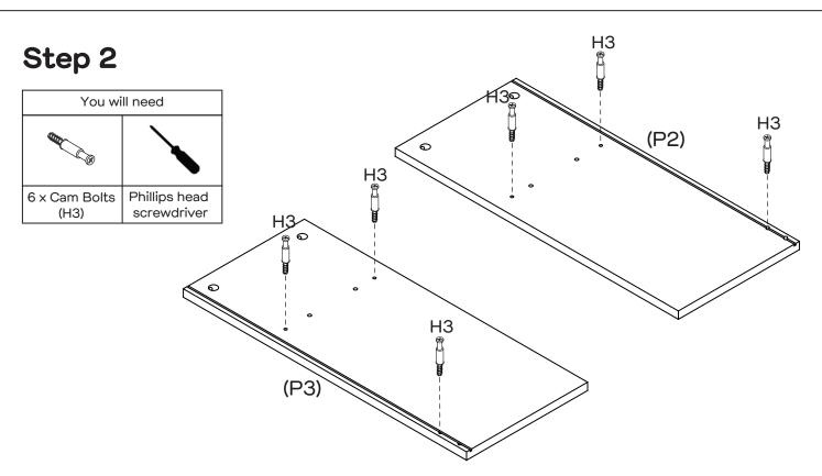
Secure 3 x Cam Bolts (H3) to Left Side Panel (P2) and 3 x Cam Bolts (H3) to Right Side Panel (P3) by tightening with the Phillips Head Screwdriver.
