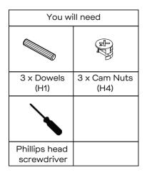
Insert 3 x Dowels (H1) & 3 x Cam Nuts (H4) into Shelf panel (P6) and Rail (P12). Attach Right Side panel (P3) to Shelf panel (P6) and Rail (P12), secure by tightening Cam Nuts (H4) with a Phillips Head Screwdriver.
