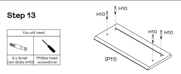
Attach 4 x Small Cam Bolts (H10) to Drawer Front (P11) by tightening with the Phillips Head Screwdriver. Repeat steps for the second drawer.
