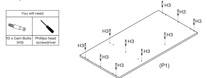
Attach 10 x Cam Bolts (H3) to Top Panel (P1) by tightening with the Phillips Head Screwdriver.
