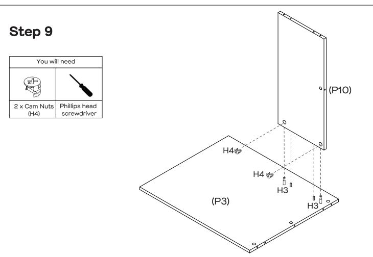
Insert 2 x Cam Nuts (H4) into Back Panel (P10). Rotate the cam nuts so the arrows point towards the incoming cam bolts. Attach Back Panel (P10) to Right Side Panel (P3) by tightening cam nuts with the Phillips Head Screwdriver.
