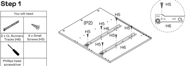
Attach 2 x CL Runner Tracks (H6) to Left Side Panel (P2) with 6 x Small Screws (H5) by tightening with the Phillips Head Screwdriver.
