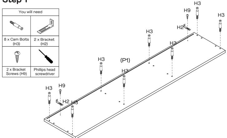
Secure 8 x Cam Bolts (H3) to Top Panel (P1) by tightening with the Phillips Head Screwdriver. Attach 2 x Brackets (H2) to Top Panel (P1) with 2 x Bracket Screws (H9) by tightening with the Phillips Head Screwdriver.
