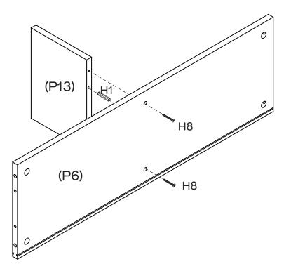
Insert 2 x Dowels (H1) into Shelf panel (P6), attach to Divider panel (P13) and secure with 2 x Large Screws (H8) by tightening with a Phillips Head Screwdriver.
