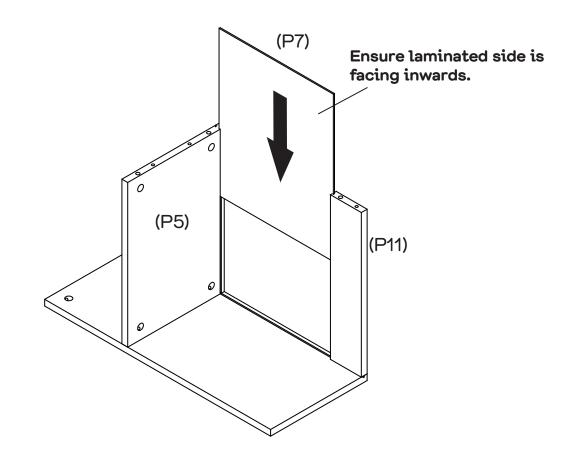
Slide Back panel (P7) into the grooves of the Shelf panel (P5) and Rail (P11) as shown.
