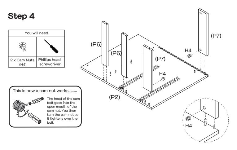
Insert 1 x Cam Nut (H4) into each Rail (P7x2). Rotate the cam nuts so the arrows point towards the incoming cam bolts. Attach Rails (P7x2) to the Left Side Panel (P2) by tightening the cam nuts with the Phillips Head Screwdriver. Attach Rails (P6x2) to Left Side Panel (P2) as shown.
