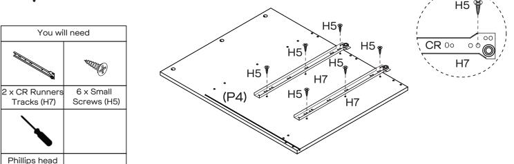
Attach 2 x CR Runner Tracks (H7) to Divider (P4) with 6 x Small Screws (H5) by tightening with the Phillips Head Screwdriver.
