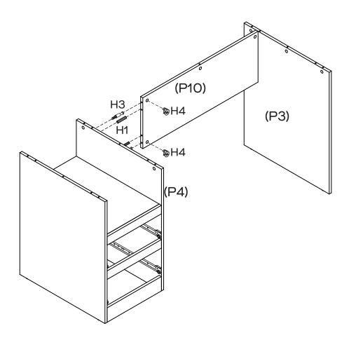
Attach 2 x Cam Bolts (H3) to Divider Panel (P4) by tightening with the Phillips Head Screwdriver. Insert 2 x Dowels (H1) and 2 x Cam Nuts (H4) into Back Panel (P10). Rotate the cam nuts so the arrows point towards the incoming cam bolts. Attach Back Panel (P10) to Divider Panel (P4) by tightening cam nuts with the Phillips Head Screwdriver.
