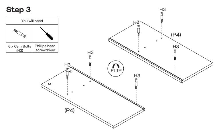
Secure 3 x Cam Bolts (H3) to Divider Panel (P4) by tightening with the Phillips Head Screwdriver. Flip the Divider Panel (P4) over and secure another 3 x Cam Bolts (H3) to the other side by tightening with the Phillips Head Screwdriver.
