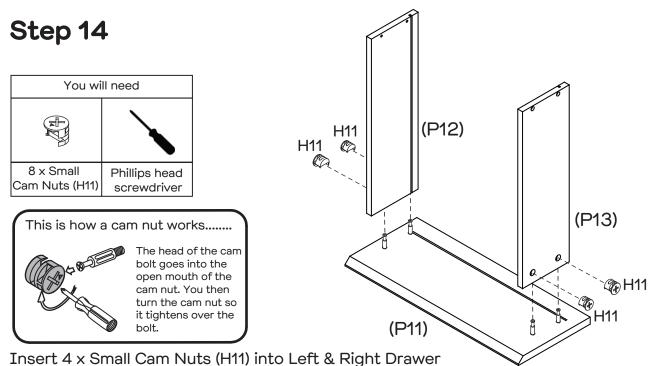
Sides (P12&P13). Rotate the cam nuts so the arrows point towards the incoming cam bolts. Attach Left & Right Drawer Sides (P12&P13) to the Drawer Front (P11) by tightening cam nuts with the Phillips Head Screwdriver. Repeat steps for the second drawer.
