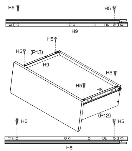
Attach 1 x DL Runner (H8) to the bottom of Left Drawer Side (P12) and 1 x DR Runner (H9) to the bottom of Right Drawer Side (P13) with 4 x Small Screws (H5) by tightening with the Phillips Head Screwdriver. Repeat steps for the second drawer
