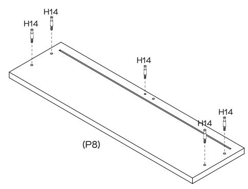
Attach 5 x Small Cam Bolts (H14) to Drawer Front (P8) as shown by tightening with the Phillips Head Screwdriver.
