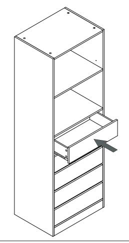
Gently insert the assembled drawers into the unit by carefully lining up the drawer runners with the drawer runner tracks.
