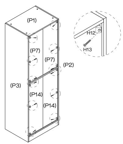
Secure Back Panels (P7  $\times$  2 & P14  $\times$  2) in place with 12  $\times$  Wedges (H12) and 12  $\times$  Wedge Screws (H13) by tightening with the Phillips Head Screwdriver.
