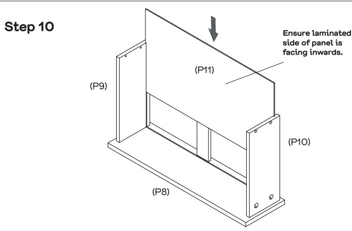
Slide Drawer Base (P11) into the grooves of Left & Right Drawer Sides (P9 & P10) and Drawer Front (P8).
