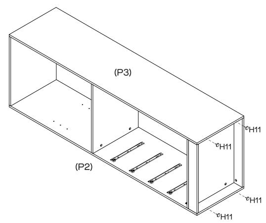
Secure 4 x Plastic Glides (H11) to the bottom of Left & Right Side Panels (P2 & P3) as shown using the Hammer.
