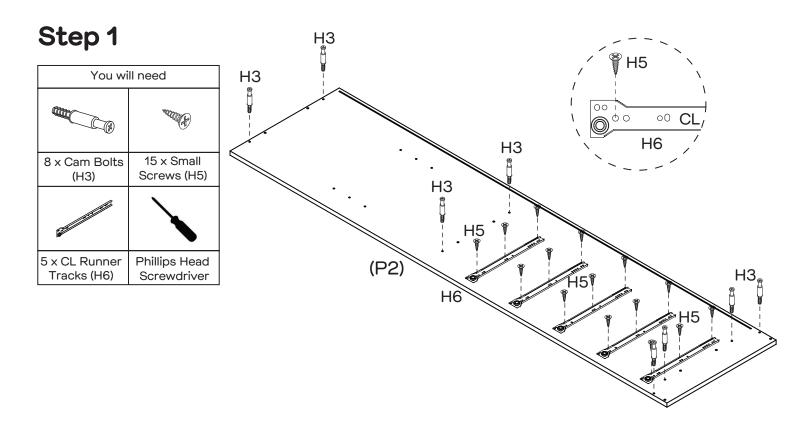
Attach 8 x Cam Bolts (H3) to Left Side Panel (P2) as shown by tightening with the Phillips Head Screwdriver. Attach  $5 \times CL$  Runner Tracks (H6) to Left Side Panel (P2) with  $15 \times Small$  Screws (H5) by tightening with the Phillips Head Screwdriver.
