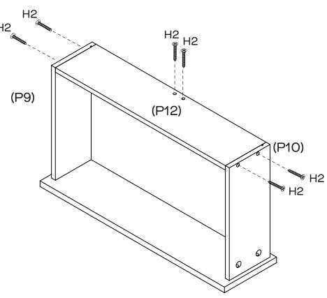
Attach Drawer Back (P12) to Left & Right Drawer Sides (P9 & P10) and Support Rail (P13) with 6 x Long Screws (H2) by tightening with the Phillips Head Screwdriver. Ensure the drawer base lines up with the grooves all the way around the drawer before securing.
