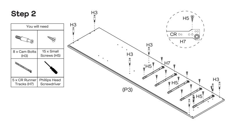
Attach 8 x Cam Bolts (H3) to Right Side Panel (P3) as shown by tightening with the Phillips Head Screwdriver. Attach  $5 \times CR$  Runner Tracks (H7) to Right Side Panel (P3) with 15 x Small Screws (H5) by tightening with the Phillips Head Screwdriver.
