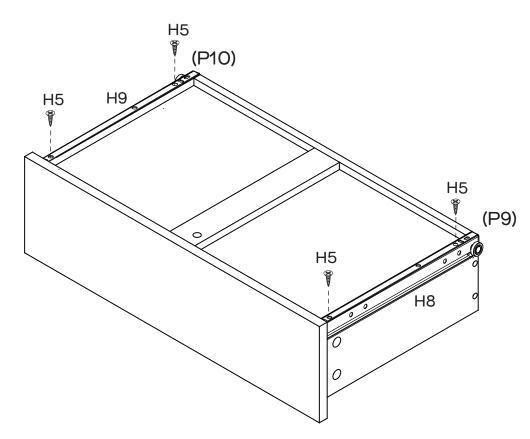
Attach 1 x DL Runner (H8) to the bottom of Left Drawer Side (P9) and 1 x DR Runner (H9) to the bottom of Right Drawer Side (P10) with 4 x Small Screws (H5) by tightening with the Phillips Head Screwdriver.
