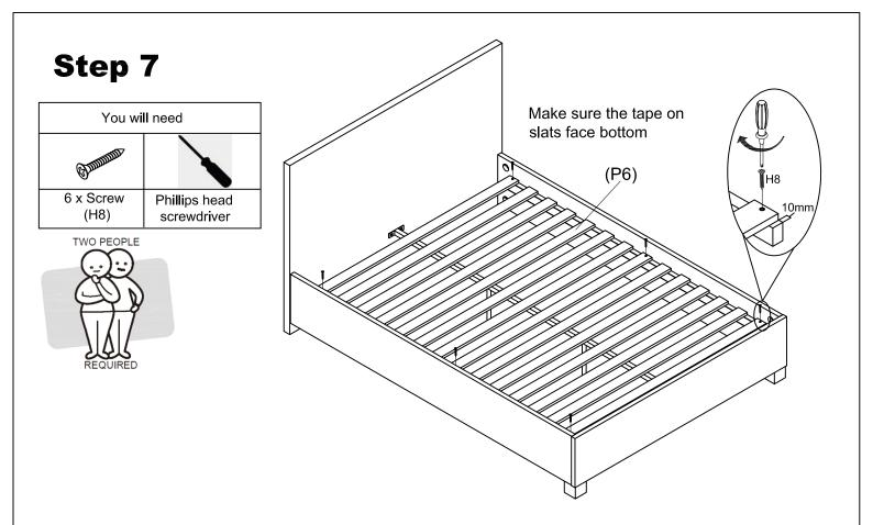
Key Slats edge is 10MM distance to the Siderail support end . Attached Slats (P6) onto the Side Rail (P3) by using 6 x Screw (H8) as shown.
