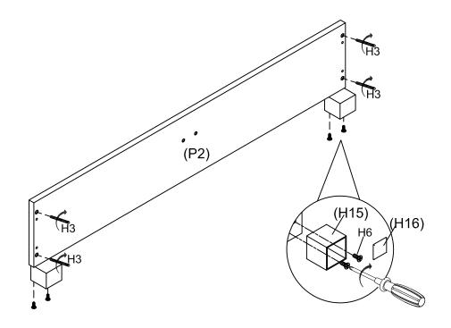
Screw 4 x Bolt (H3) onto Footboard (P2) Attch 2 x Legs (H15) to Footboard (P2) by using 4 x Bolt (H6), and tighten with a Phillips Head Screwdriver. Then insert the Leg cap (H16) as shown.
