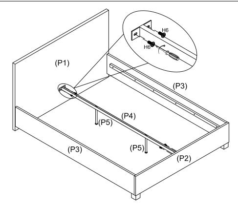
Attach Centre Rail (P4) to the Headboard (P1) and Footboard (P2) by using 4 x Bolt(H6)
