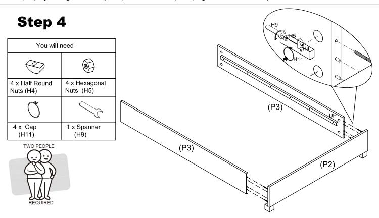
Attach 2 x Side Rails (P3) to Footboard (P2) by using 4 x Hexagonal Nuts (H5) 4 x Halfround Nut (H4) as show, tighten with a Spanner (H9), insert 4 x Caps (H11)
