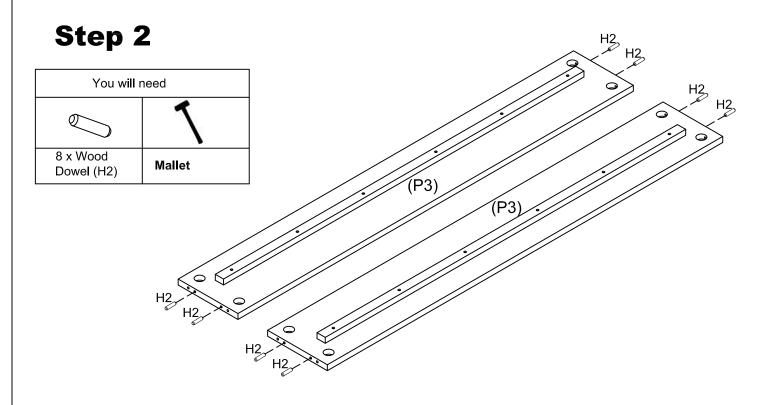
Using the Mallet if needed, Insert 8 x Wooden Dowels (H2) to the hole on Side Rails (P3) as shown.
