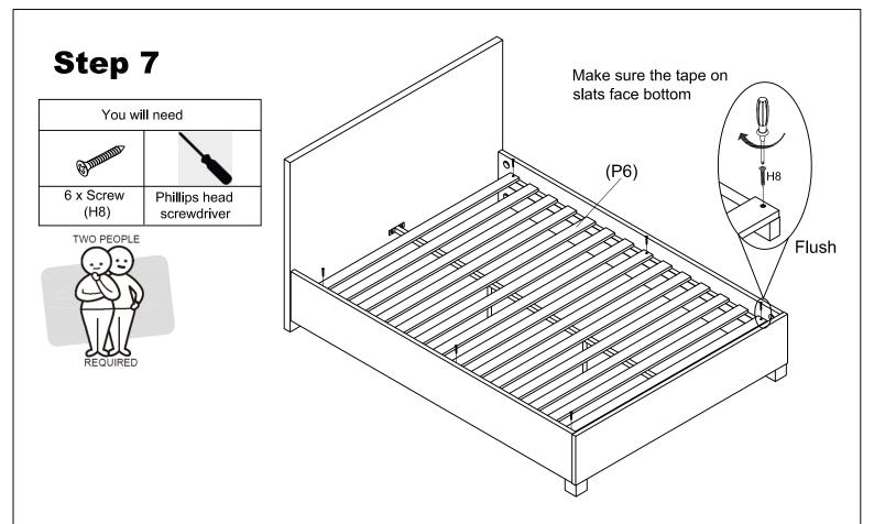
Key Slats side edge is flush with Siderail support end. Attached Slats (P6) onto the Side Rail (P3) by using 6 x Screw (H8) as shown.
