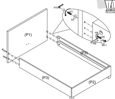
Attach Headboard (P1)to Side Rail (P3)by using 4 x Bolt (H1) 4 x Hexagonal Nuts (H5)4 x Half Round Nut (H4)and 4 x Washer (H7) as shown, tigten with a Spanner (H9) and Allen Key (H10), and insert 4 x Caps (H11)
