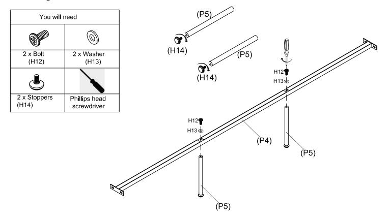
Insert the 2 x Stoppers (H14)to the 2 x Support legs (P5). Attach 2 x Support Legs (P5) to Centre Rail (P4) by using 2 x Bolt (H12) and Washer (H13) tighten with a Phillips Head Screwdriver.
