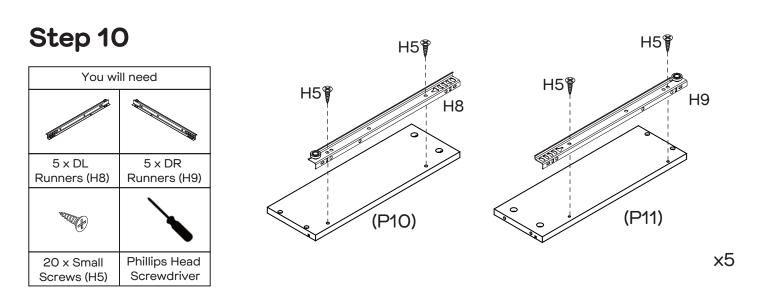
Attach 5 x DL Runners (H8) to the bottom of Left Drawer Sides (P10x5) and 5 x DR Runners (H9) to the bottom of Right Drawer Sides (P11x5) with 20 x Small Screws (H5) by tightening with the Phillips Head Screwdriver.
