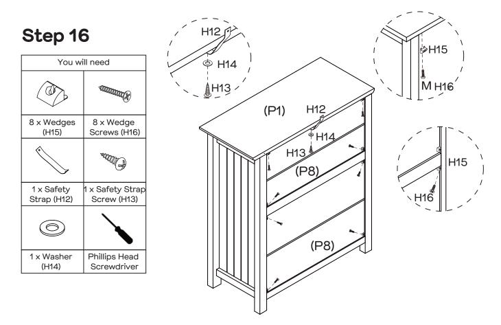
Secure Back Panels (P8  $\times$  4) in place with 8  $\times$  Wedges (H15) using 8  $\times$  Wedge Screws (H16) by tightening with the Phillips Head Screwdriver. Use 1  $\times$  Safety Screw (H13) and 1  $\times$  Washer (H14) to connect 1  $\times$  Safety Strap (H12) on Top Panel (P1).
