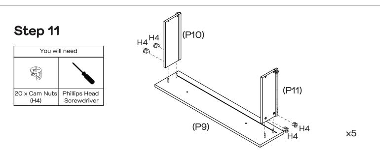
Insert 20 x Cam Nuts (H4) into Left & Right Drawer Sides (P10x5&P11x5) as shown. Rotate the cam nuts so the arrows point towards the incoming cam bolts. Attach Left & Right Drawer Sides (P10x5&P11x5) to Drawer Fronts (P9x5) by tightening the cam nuts with the Phillips Head Screwdriver.
