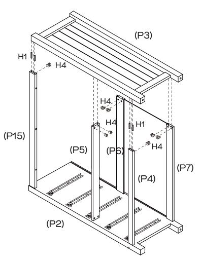
Insert 8 x Cam Nuts (H4) into the holes of Rails (P4&P5&P6&P7&P15). Rotate the cam nuts so the arrow points towards the incoming cam bolts. Attach Rails (P4&P5&P6&P7&P15) to Right Side Panels (P3) by tightening with the Phillips Head Screwdriver.
