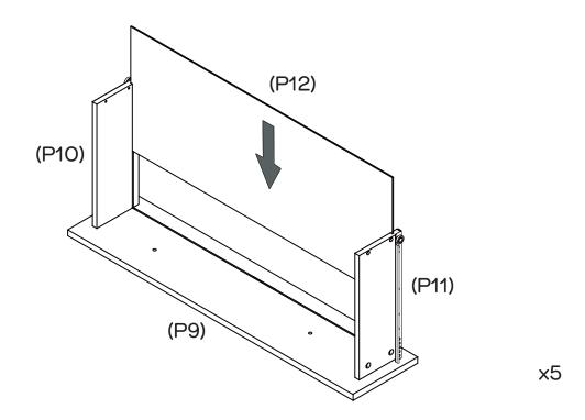
Slide Drawer Bases (P12x5) into the grooves of Left & Right Drawer Sides (P10x5&P11x5).
