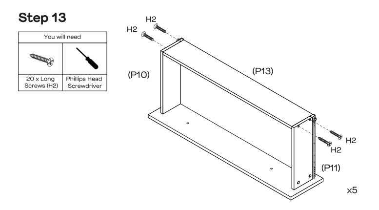
Attach Drawer Backs (P13x5) to Left & Right Drawer Sides (P10x5&P11x5) with 20 x Long Screws (H2) by tightening with the Phillips Head Screwdriver. Ensure the Drawer Base lines up with the grooves the whole way around the drawer before securing.
