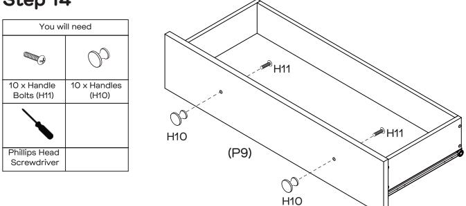
Attach 10 x Handles (H10) to Drawer Fronts (P9x5) with 10 x Handle Bolts (H11) by tightening with the Phillips Head Screwdriver.
