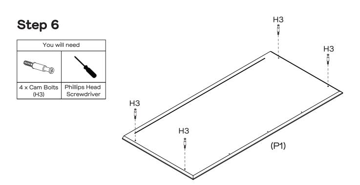
Attach 4 x Cam Bolts (H3) to Top Panel (P1) by tightening with the Phillips Head Screwdriver.
