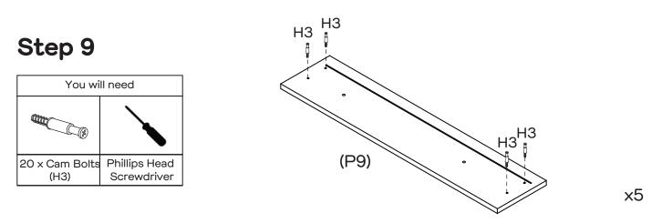
Attach 20 x Cam Bolts (H3) to Drawer Fronts (P9x5) by tightening with the Phillips Head Screwdriver.
