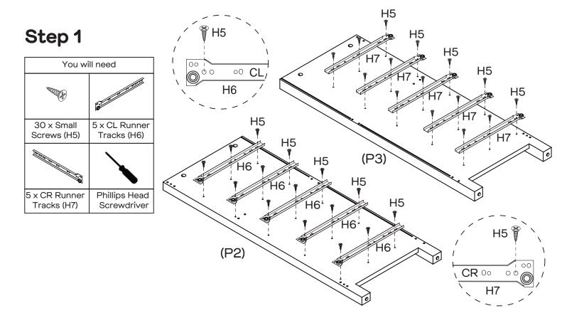
Attach 5x CL Runner Tracks (H6) and 5 x CR Runner Tracks (H7) to Left & Right Side Panels (P2&P3) with 30 x Small Screws (H5) by tightening with the Phillips Head Screwdriver.
