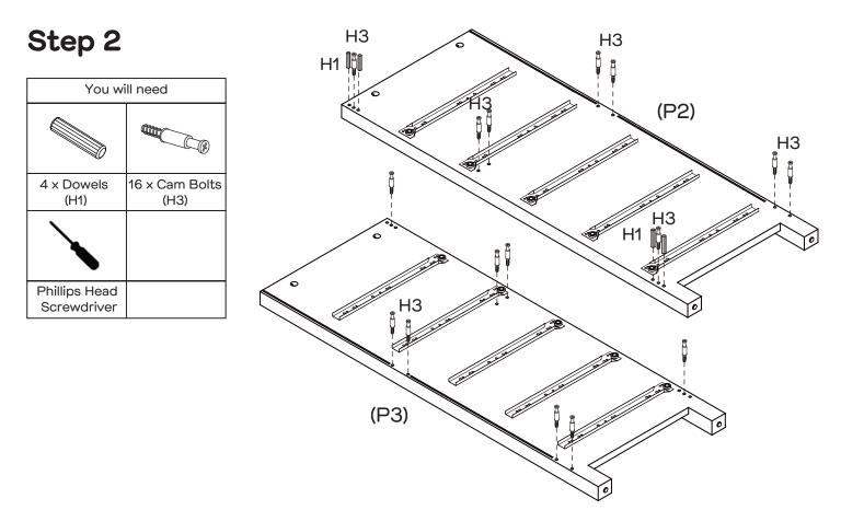
Insert 4x Dowels (H1) into Left (P2) as shown. Attach 16 x Cam Bolts (H3) to Left & Right Side Panels (P2&P3) by tightening with the Phillips Head Screwdriver.
