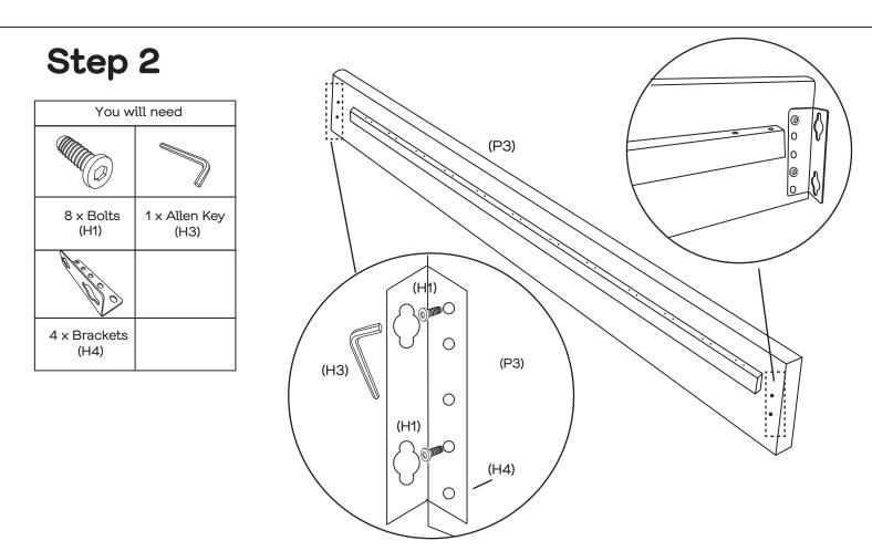
Attach the 4 x brackets (H4) to the ends of the side rails (P3) as shown. Screw in 2 x bolts (H1) into each bracket with the allen key (H3). Ensure to fully tighten all bolts.
