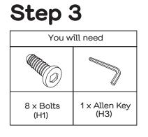
Install 4 x bolts (H1) into the headboard (P1) and footboard (P2) by using the allen key (H3) as shown, do not fully tighten the bolts and keep them 8mm loose.
