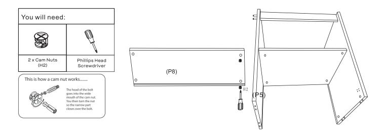
Insert 2 x Cam Nuts(H2) into Long Shelf(P8) as shown. Rotate the cam nuts so the arrows point towards the incoming cam bolts.
