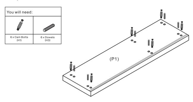
Insert 6 x Dowels(H3) into Top Panel(P1) and secure 6 x Cam Bolts(H1) into Top Panel(P1) by tightening with the Phillips Head Screwdriver.
