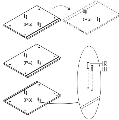
Insert 2 x Dowels(H3) into Right Panel(P3) and secure 2 x Cam Bolts(H1) to Right Panel(P3) by tightening with a Phillips Head Screwdriver. Repeat for Left Panel (P4)
