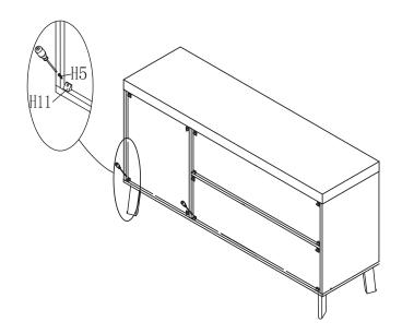
Insert 12 x Wedges(H11) into all corners of the back of the assembled unit as shown. Secure the 12 x Wedges (H11) to the assembled unit using 12 x Short Screws (H5), tightening with the Phillips Head Screwdriver.
