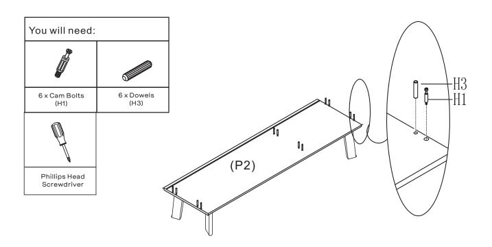
Insert 6 x Dowels (H3) into Bottom Panel (P2). Secure 6 x Cam Bolts (H1) into Bottom Panel (P2), tightening using a Phillips Head Screwdriver.
