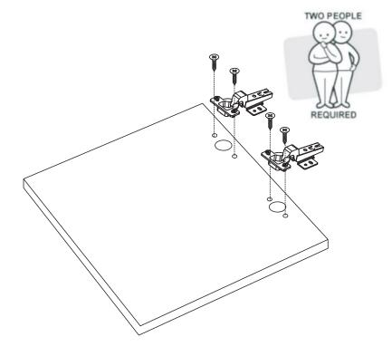
Attach 2 x hinges (H4) to 1 x right door (P13) using 4 x short screws (H5) as shown. Tighten using a phillips head screwdriver. Repeat this step for the other right door (P13) and the left door (P12).
