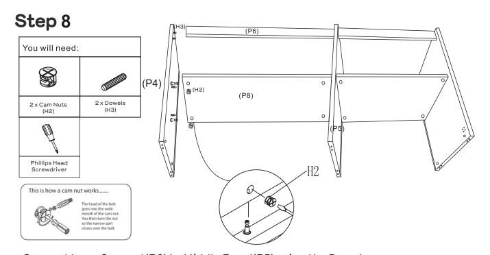
Connect Long Support(P6) to Middle Panel(P5) using the Dowels (H15) on the Middle Panel (P5). Insert 2 x Dowels(H3) into Left Panel(P4). Insert 2 x Cam Nuts(H2) into Long Shelf(P8) as shown. Rotate the cam nuts so the arrows point towards the incoming cam bolts. Align the Left Panel (P4) with the Long Support (P6) and Long Shelf (P8) as shown.
