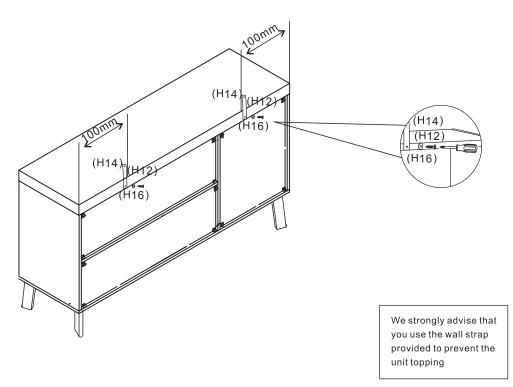
Use 2 x Washers (H16) and 2 x Long Screws (H12) to secure the Wall Strap (H14) to the middle of the Top Panel (P1) as shown. Tighten using the Phillips Head Screwdriver.
