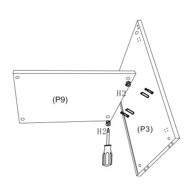
Insert 2 x Cam Nuts(H2) into Short Shelf(P9) as shown. Rotate the cam nuts so the arrows point towards the incoming cam bolts.
