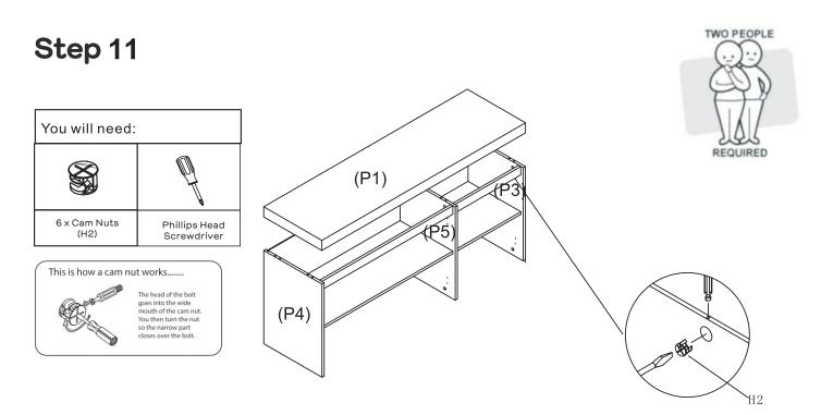
Insert 6 x Cam Nuts(H2) into Panel(P3&P4&P5) as shown.Rotate the cam nuts so the arrows point towards the incoming cam bolts. With assistance, attach the Top Panel (P1) to the assembled frame (P3, P4, P5) as shown. Attach together by tightening the Cam Nuts (H2) on the assembled frame (P3, P4, P5) by turning clockwise using the Phillips Head Screwdriver.
