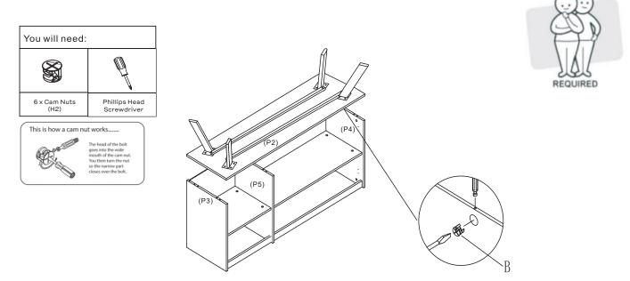
Insert 6 x Cam Nuts(H2) into Panel(P3&P4&P5) as shown. Rotate the cam nuts so the arrows point towards the incoming cam bolts. With assistance, attach the Bottom panel (P2) to the assembled frame (P3, P4, P5) as shown. Attach together by tightening the Cam Nuts (H2) on the assembled frame (P3, P4, P5) by turning clockwise using the Phillips Head Screwdriver.
