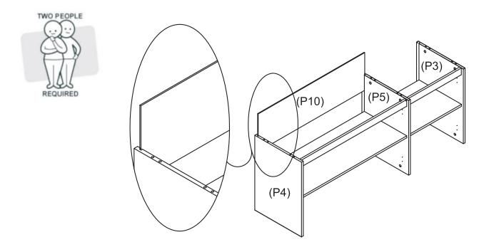
With assistane, carefully turn the assembled frame upright. Slide 1 x Long Back Panel (P10) through the grooves on the Left Panel (P4) and Middle Panel (P5) as shown.
