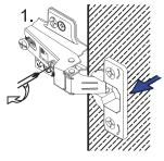
MOVE DOOR **OUTWARD** by turning this screw clockwise
