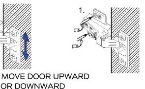
**STEP 16.2** Adjust the door panels upward or downward
