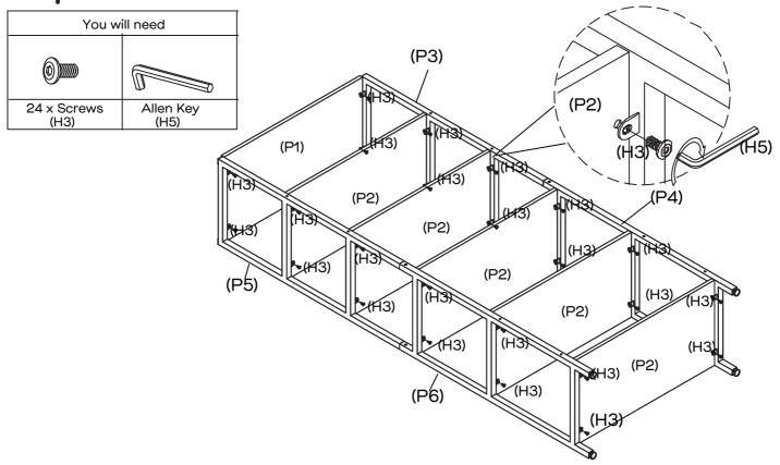
Secure Top Panel (P1) and Shelf Panels (P2x5) to Top & Lower Left/Right Frames (P3,P4,P5&P6) with 24 x Screws (H3) as shown by tightening with the Allen Key (H5). fantasticfurniture.com.au
