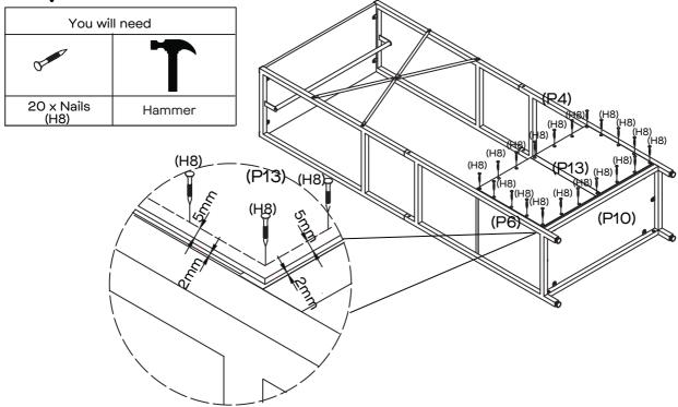
Secure Back Panel (P13) to the back of the partially assembled drawer unit as shown with 20 x Nails, approximately 5mm from the edge, using the Hammer. Ensure the Back Panel is sitting square in the unit before securing, with about 2mm around each edge.
