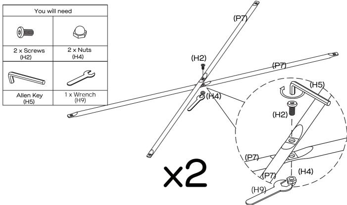
Secure Back Supports (P7×2) together as shown with 1 x Nut (H4) and 1 x Screw (H2) by tightening with the Allen Key (H5) and Wrench (H9).
