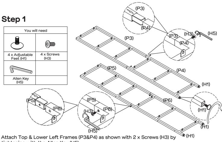
tightening with the Allen Key (H5).
