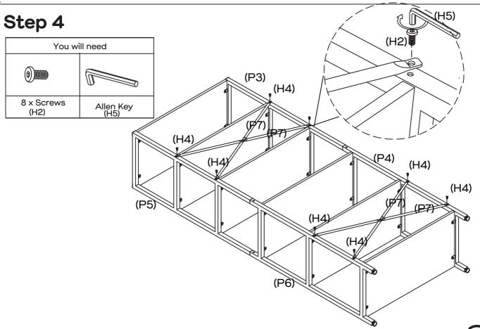
Attach Back Supports (P7x4) to Top & Lower Left/Right Frames (P3,P4,P5&P6) as shown with 8 x Screws (H2) by tightening with the Allen Key (H5). fantasticfurniture.com.au
