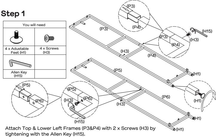
Repeat steps for Top & Lower Right Frames (P5&P6). Secure 4 x Adjustable Feet (H1)to the bottom of Lower Left & Right Frames (P4&P6) as shown.
