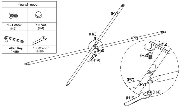
Secure Back Supports (P7x2) together as shown with  $1 \times \text{Nut}$  (H4) and  $1 \times \text{Screw}$  (H2) by tightening with the Allen Key (H15) and Wrench (H19).
