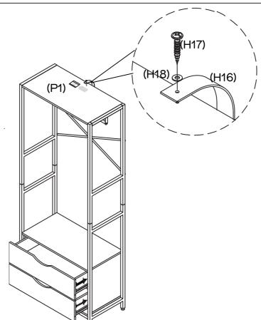
Attach the Wall Strap (H16) to Top Panel (P1) with 1 x Washer (H18) and 1 x Wall Strap Screw (H17) by tightening with the Phillips Head Screwdriver.
