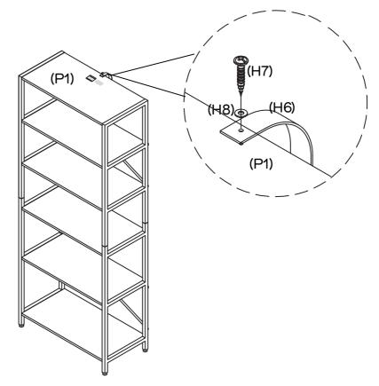
Attach the Wall Strap (H6) to Top Panel (P1) with 1 x Washer (H8) and 1 x Wall Strap Screw (H7) by tightening with the Phillips Head Screwdriver.
