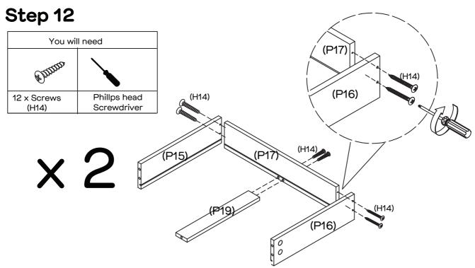
Secure Left & Right Drawer Sides (P15&P16) to Back Panel (P17) with 4 x Screws (H14) by tightening with the Phillips Head Screwdriver. Attach Drawer Support Panel (P19) to Back Panel (P17) with 2 x Screws (H14) by tightening with the Phillips Head Screwdriver. Repeat steps for the second Drawer.
