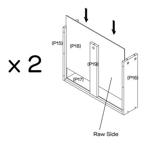
Slide Drawer Base (P18) into the grooves of Left & Right Drawer Sides (P15&P16) and Back Panel (P17).
