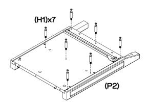
Attach  $7 \times \text{large cam bolts}$  (H1) to left side (P2) using a phillips head screwdriver.
