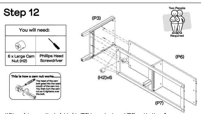
With assistance, attach right side (P3) to centre board (P6) and bottom frame (P7). Insert 6 x large cam nuts (H2) into centre board (P6) and bottom frame (P7). Using a phillips head screwdriver, rotate the cam nuts (H2) so the arrows point towards incoming cam bolts. Turn clockwise to lock.
