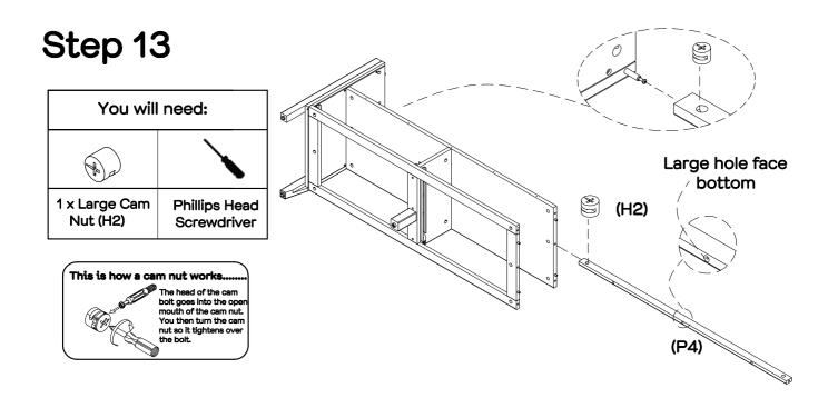
Attach top panel rail (P4) to the assembled frame as shown. Insert 1 x large cam nut (H2) into top panel rail (P4). Using a phillips head screwdriver, rotate the cam nut so the arrow points towards incoming cam bolt. Turn clockwise to lock.
