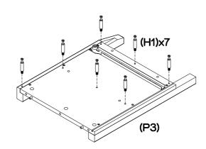
Attach  $7 \times 1$  large cam bolts (H1) to right side (P3) using a phillips head screwdriver.
