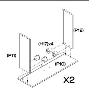
Attach 1 x left drawer side (P11) and 1 x right drawer side (P12) to 1 x drawer front (P10), ensuring the grooves on each panel align. Insert 4 x small cam nuts (H17) into the drawer sides (P11, P12). Using a phillips head screwdriver, rotate so the arrow on the cam nut 9 (H17) points towards incoming cam bolts. Turn clockwise to lock. Repeat this step for the other drawer.
