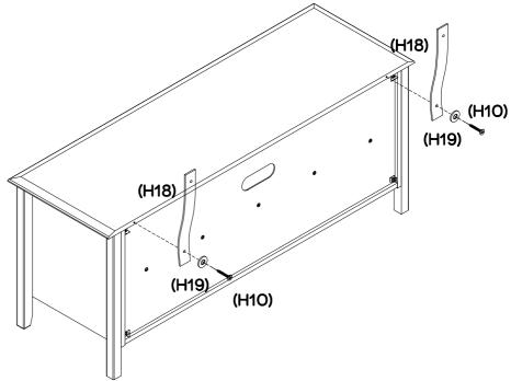
Attach 2 x wall straps (H18) to the back of the top panel (P1) using  $2 \times \text{large}$  screws (H10) and  $2 \times \text{washers}$  (H19).
