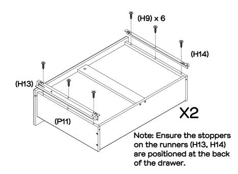
Attach 1 x left runner (H13) to left drawer side (P11), and 1 x right runner (H14) to right drawer side (P12) using  $6 \times 8$  x small screws. Tighten using a phillips head screwdriver. Repeat this step for the other drawer.
