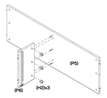
Attach the centre board (P6) to the shelf (P5) as shown. Insert  $3 \times 1$  large cam nuts (H2) into centre board (P6). Using a phillips head screwdriver, rotate the cam nuts so the arrow points towards the incoming cam bolt. Turn clockwise to lock.
