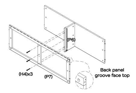
Attach the bottom frame (P7) to the centre board (P6) using  $3 \times 1$  large screws (H5), tightening with a phillips head screwdriver.
