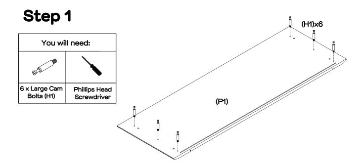
Attach 6 x large cam bolts (H1) to top panel (P1) using a phillips head screwdriver.
