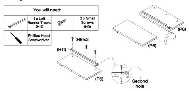
Turn over the centre board (P6) and attach 1  $\times$  left runner track (H11) using 3  $\times$  small screws (H9), tightening with a phillips head screwdriver. Ensure the srews are inserted into the holes shown in the image above.
