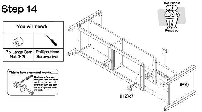
With assistance, attach left side (P2) to centre board (P6) and bottom frame (P7). Insert 7 x large cam nuts (H2) into centre board (P6),bottom frame (P7) and top panel rail (P4). Using a phillips head screwdriver, rotate the cam nuts (H2) so the arrow points towards incoming cam bolt. Turn clockwise to lock. fantasticfurniture.com.au
