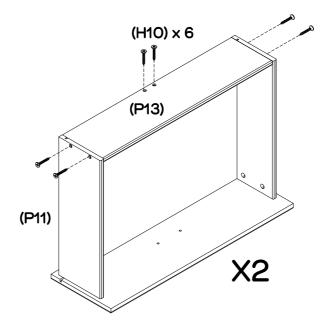
Attach 1  $\times$  drawer back panel (P13) to drawer sides (P11, P12) and drawer support rail (P15) using 6  $\times$  medium screws (H10). Repeat this process for the other drawer.
