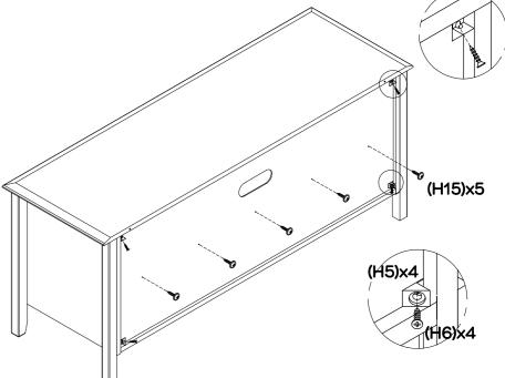
Attach back panel (P9) to shelf (P5) using  $5 \times back$  panel screws (H15), tightening with a phillips head screwdriver. Attach  $4 \times back$  panel supports (H5) to each corner of the unit. Secure using  $4 \times back$  panel support screws (H6), tightening with a phillips head screwdriver. fantasticfurniture.com.au
