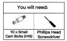
Attach  $5 \times \text{small cam bolts}$  (H16) to  $1 \times \text{drawer front}$  (P10) using a phillips head screwdriver. Repeat this step for the other drawer front (P10).
