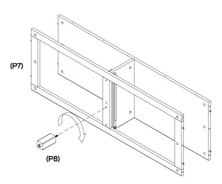
Attach middle foot (P8) to the bottom frame (P7) by turning clockwise to clock.
