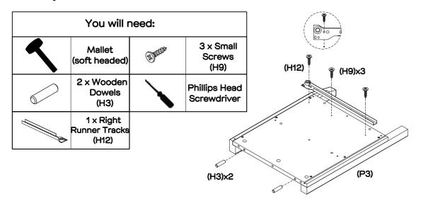
Insert 2 x wooden dowels (H3) into right side (P3). Attach 1 x right runner track (H12) to right side (P3) using 3 x small screws (H9), tightening with a phillips head screwdriver. Ensure you insert the screws (H9) into the holes on the track (H12) as shown.
