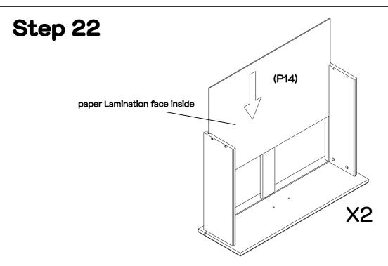
Slide 1 x drawer base (P14) into the grooves on the drawer sides (P11, P12) and drawer front (P10). Repeat this process for the other drawer.
