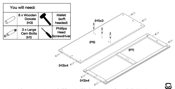
Insert 8  $\times$  wooden dowels (H3) into shelf (P5) and bottom frame (P7). Attach 3  $\times$  large cam bolts (H1) to shelf (P5), using a phillips head srewdriver.
