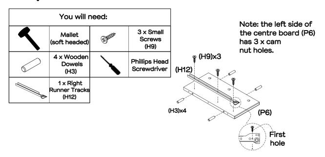
Insert 4  $\times$  wooden dowels (H3) into centre board (P6). Attach 1  $\times$  right runner (H12) to the left side of centre board (P6) using 3  $\times$  small screws (H9), tightening with a phillips head screwdriver. Ensure the screws are inserted into the holes shown in the image above.
