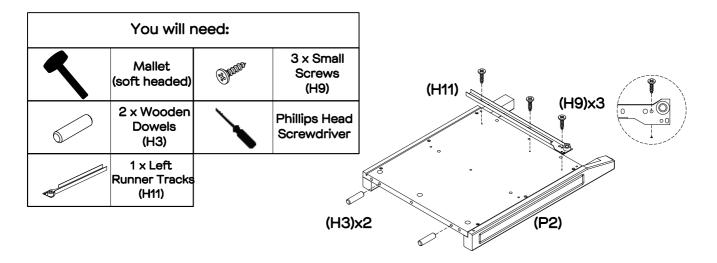
Insert 2 x wooden dowels (H3) into left side (P2).
