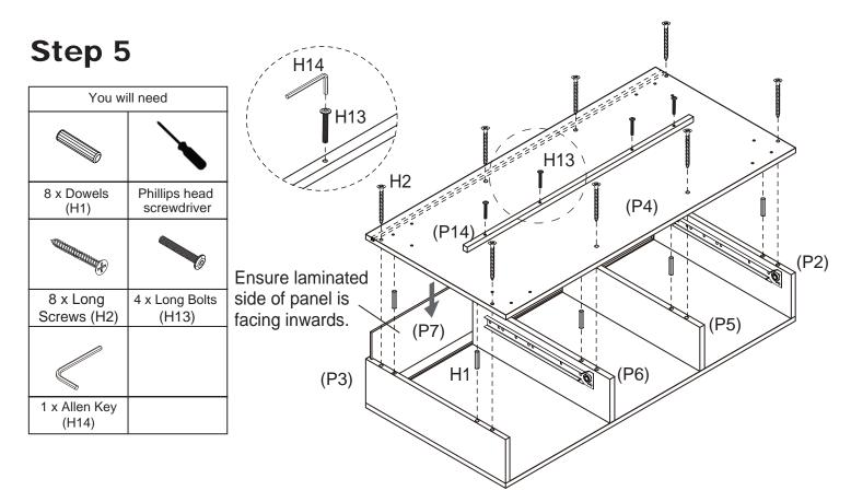
Slide back panel (P7) into the groove of left side panel (P2) and right side panel (P3). Attach rail (P14) to bottom panel (P4) secure with 4 x long bolts (H13). Tighten with an Allen key (H14). Attach bottom panel (P4) to the main unit with 8x dowels (H1), and secure with 8x long screws (H2). Tighten with a Phillips head screwdriver.
