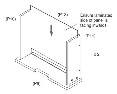
Slide drawer base (P13) into the groove of drawer sides (P10, P11). Repeat for second drawer.
