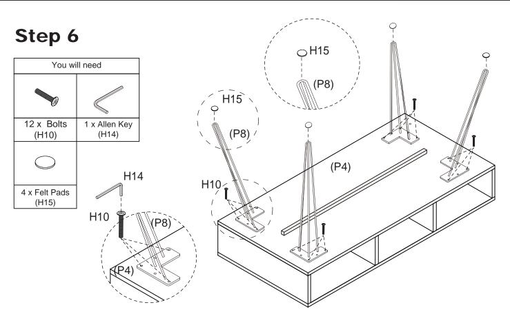
Attach 4x legs (P8) to bottom panel (P4) and secure with 12 x bolts (H10). Tighten with an Allen key (H14). Apply 4 x felt pads (H15) to bottom of legs (P8) as shown.
