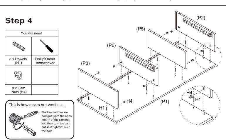
Attach left side panel (P2) ,right side panel (P3) ,left divider (P5) and right divider (P6) to top panel (P1) with 8x dowels (H1),and secure with 8x cam nuts (H4). Tighten with a Phillips head screwdriver.
