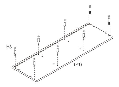
Attach 8 x cam bolts (H3) to top panel (P1) as shown. Tighten with a Phillips head screwdriver.
