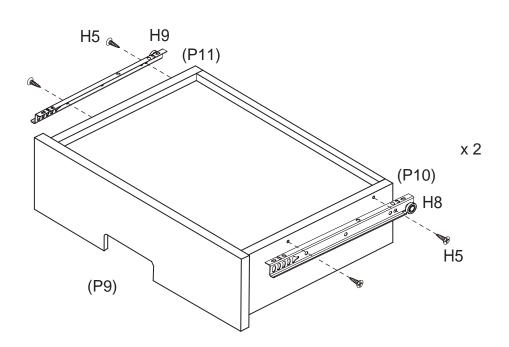
Attach 1 x DL runner (H8) to left drawer side (P10) and 1 x DR runner (H9) to right drawer side (P11) with 4 x small screws (H5). Tighten screws using a Phillips head screwdriver. Repeat for second drawer.
