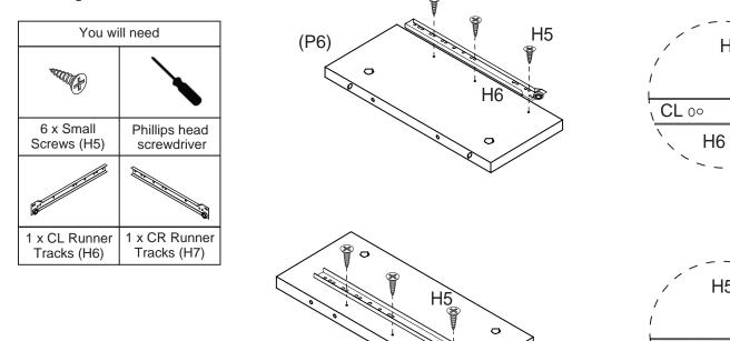
Attach 1 x CR runner tracks (H7) to left divider (P5) with 3 x small screws (H5). Attach 1 x CL runner tracks (H6) to right divider (P6) with 3 x small screws (H5). Tighten with a Phillips head screwdriver.
