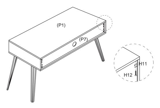
Secure Back Panel (P7) in place with 4 x wedges (H11) using 4 x screws (H12).
