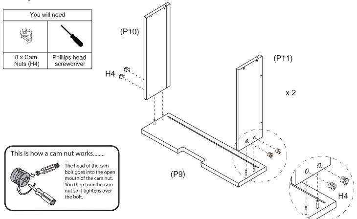
Attach drawer sides (P10, P11) to drawer front (P9). Insert 4 x cam nuts (H4) into the holes of drawer sides (P10, P11). Make sure the opening on cam nuts point towards the incoming cam bolts. Tighten the cam nuts using a Phillips head screwdriver. Repeat for second drawer.
