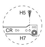
Attach 1 x CL runner tracks (H6) to left side panel (P2) with 3 x small screws (H5). 1 x CR runner tracks (H7) to right side panel (P3) with 3 x small screws (H5). Tighten with a Phillips head screwdriver.
