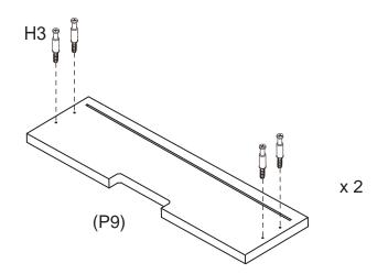
Screw 4 x cam bolts (H3) into drawer front (P9) with a Phillips head screwdriver. Repeat for second drawer.
