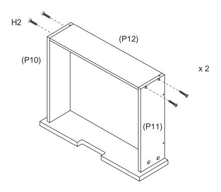
Attach drawer back (P12) to drawer sides (P10, P11) with 4 x long screws (H2), make sure that the groove lines up the whole way around the drawer. Tighten screws using a Phillips head screwdriver. Repeat for second drawer.
