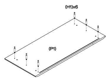
Attach 6  $\times$  large cam bolts (H1) to top panel (P1) using a phillips head screwdriver.
