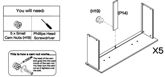
Attach 1 x drawer support rail (P14) to 1 x drawer front (P9), ensuring the side with the cam nut holes faces outwards. Insert 1 x small cam nut (H19) into the drawer support rail (P14). Using a phillips head screwdriver, rotate the cam nut so the arrows faces incoming cam bolt. Turn clockwise to lock. Repeat this process for the other 4 x support rails (P14).
