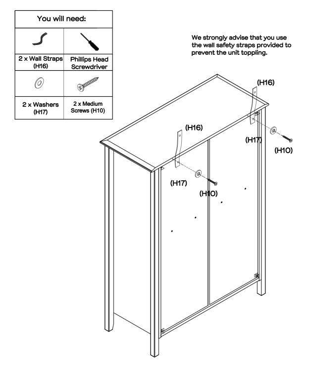
Attach 2 x wall straps (H16) to the back of top panel (P1) using 2 x medium screws (H1O) and 2 x washers (H17), tightening using a phillips head screwdriver.
