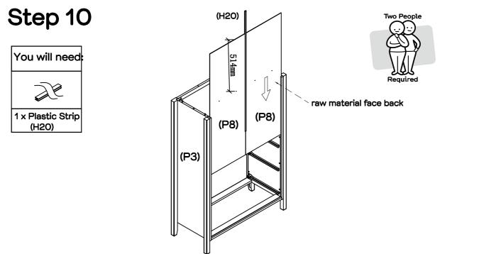
With assistance, carefully turn the unit upright. Slide the 2 x back panels (P8) into the grooves on the side panels (P2, P3) and rear lower rail (P6). Ensure the informative label is positioned as shown. Insert the plastic strip (H2O) between the 2 x back panels (P8) as shown.
