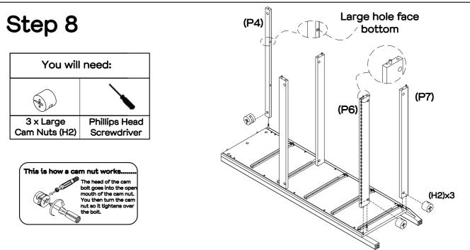
Attach front upper rail (P4) to right side (P3), ensuring the side with the cam nut hole faces inwards. Attach the rear lower rail (P6) and front lower rail (P7) to right side (P3), ensuring the sides with the cam nut holes faces outwards. Insert 3 × large cam nuts into the rails (P4, P6, P7). Using a phillips head screwdriver, rotate the cam nuts (H2) so the arrow points towards incoming cam bolts. Turn clockwise to lock. fantasticfurniture.com.au
