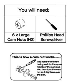
Attach top panel (P1) to unit as shown. Insert 6 x large cam nuts (H2) into the left and right side (P2, P3). Using a phillips head screwdriver, rotate the cam nuts (H2) so the arrow points towards incoming cam bolts. Turn clockwise to lock.
