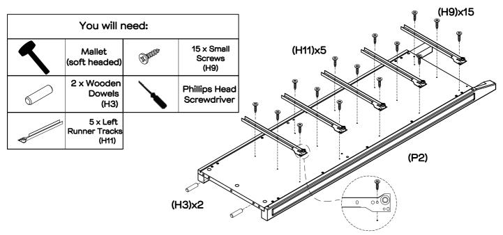
Insert 2 x wooden dowels (H3) into left side (P2). Attach 5 x left runner tracks (H11) to left side (P2) using 15 x small screws (H9), tightening using a phillips head screwdriver. Ensure the screws are inserted into the holes on the tracks (H11) as shown above.
