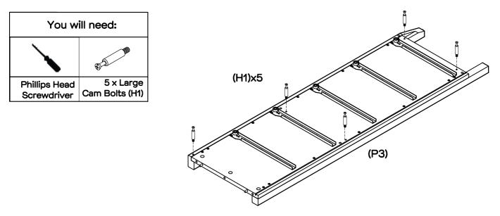
Attach  $5 \times$  large cam bolts (H1) into right side (P3) using a phillips head screwdriver.
