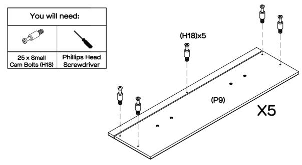
Attach 5 x small cam bolts (H18) to 1 x drawer front (P9) using a phillips head screwdriver. Repeat this step for the other 4 x drawer fronts (P9).
