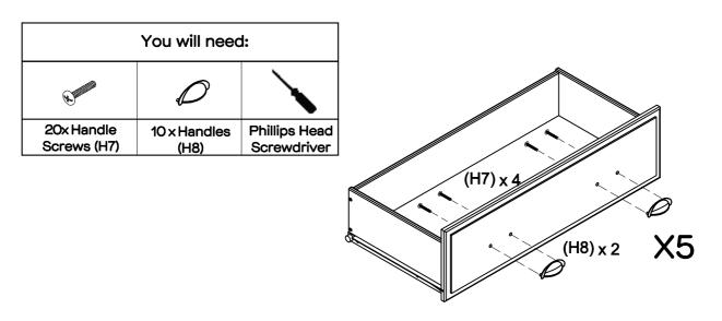
Attach 2 x handles (H8) to 1 x drawer front (P9) using 4 x handle screws (H7), tightening with a phillips head screwdriver. Repeat this process for the other  $4 \times assembled$  drawers.
