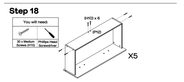
Attach 1 x drawer back panel (P12) to the side panels (P10, P11) and drawer support rail (P14) using 6 x medium screws (H10), tightening with a phillips head screwdriver. Repeat this process for the other 4 x drawer back panels (P12).
