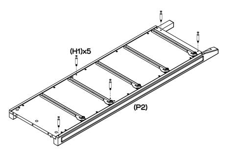
Attach 5  $\times$  large cam bolts (H1) into left side (P2) using a phillips head screwdriver.
