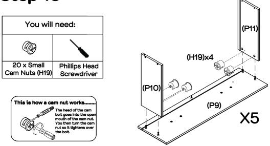
Attach 1 x drawer left side (P10) and 1 x drawer right side (P11) to 1 x drawer front (P9), ensuring the grooves on all the panels align. Insert 4 x small cam nuts (H19) into the drawer sides (P10,P11). Using a phillips head screwdriver, rotate the cam nuts so the arrow points towards the incoming cam bolts. Turn clockwise to lock.Repeat this process for the other 5 x drawer side panels (P10, P11).
