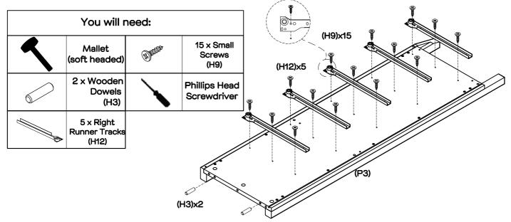
Insert 2 x wooden dowels (H3) into right side (P3). Attach 5 x right runner tracks (H12) to right side (P3) using 15 x small screws (H9), tightening using a phillips head screwdriver. Ensure the screws are inserted into the holes on the tracks (H12) as shown above.
