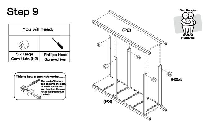
With assistance, attach left side (P2) to assembled unit. Insert  $5 \times 1$  arge cam nuts into rails (P4, P5, P6, P7). Using a phillips head screwdriver, rotate the cam nuts (H2) so the arrows point towards the incoming cam bolt. Turn clockwise to lock.
