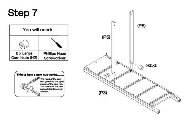
Attach 2 x middle rails (P5) to right side (P3), ensuring the sides with the cam nut holes are facing outwards. Using a phillips head screwdriver, rotate the cam nuts (H2) so the arrow points towards the incoming cam bolt. Turn clockwise to lock.
