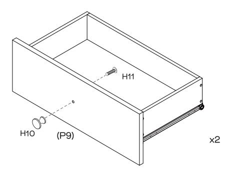
Attach 2  $\times$  Handles (H11) to Drawer Fronts (P9x2) with 2  $\times$  Handle Bolts (H10) by tightening with the Phillips Head Screwdriver.
