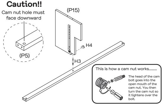
Attach 1 x Cam Bolt (H3) into Rail (P5) by tightening with the Phillips Head Screwdriver. Insert 1 x Cam Nut (H4) into the hole of Rail (P5). Rotate the cam nuts so the arrow points towards the incoming cam bolts. Attach Rails (P5) to Divider (P15) by tightening with the Phillips Head Screwdriver.
