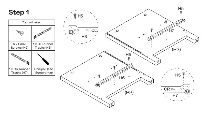
Attach 1 x CL Runner Track (H6) to Left Side Panel (P2) and 1 x CR Runner Track (H7) to the Right Side Panel (P3) with  $6 \times 8$  Small Screws (H5) by tightening with the Phillips Head Screwdriver.
