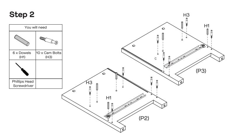
Insert 6x dowels (H1) to Left & Right Side Panels (P2&P3) as shown. Attach 10  $\times$  Cam Bolts (H3) to Left & Right Side Panels (P2&P3) by tightening with the Phillips Head Screwdriver.
