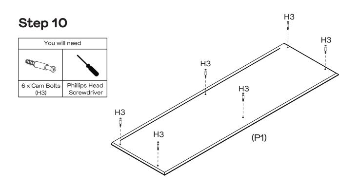
Attach 6 x Cam Bolts (H3) to Top Panel (P1) by tightening with the Phillips Head Screwdriver.
