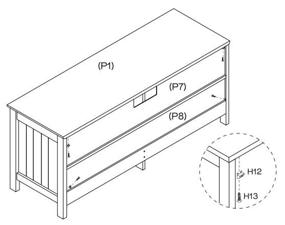
Secure Back Panels (P7 & P8) in place with 4 x Wedges (H12) using 4 x Wedge Screws (H13) by tightening with the Phillips Head Screwdriver.
