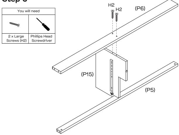
Attach Rail (P6) to Divider (P15) with 2 x Large Screws (H2) by tightening with the Phillips Head Screwdriver.
