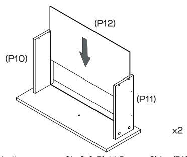
Slide Drawer Bases (P12x2) into the grooves of Left & Right Drawer Sides (P10x2&P11x2).
