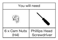
Gently stand the unit upright. Slide Back Panel (P7) into the grooves of Left & Right Side Panel (P2&P3). Insert 6 x Cam Nuts (H4) into Divider & Right & Left Side Panels (P14&P3&P2) as shown. Rotate the cam nuts so the arrows point towards the incoming cam bolts. Attach Top Panel (P1) to unit by tightening cam nuts with the Phillips Head Screwdriver.
