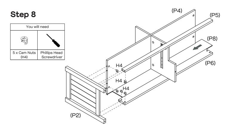
Insert 5 x Cam Nuts (H4) into the holes of Rails & Shelf Panel (P5 & P6 & P4). Rotate the cam nuts so the arrow points towards the incoming cam bolts. Attach Rails & Shelf Panel (P5 & P6 & P4) to Left Side Panel (P2) by tightening with the Phillips Head Screwdriver. Slide Back Panel (P8) into the grooves of Rail & Shelf Panel (P6&P4).
