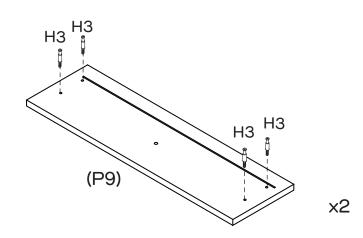
Attach 8 x Cam Bolts (H3) to Drawer Fronts (P9x2) by tightening with the Phillips Head Screwdriver.
