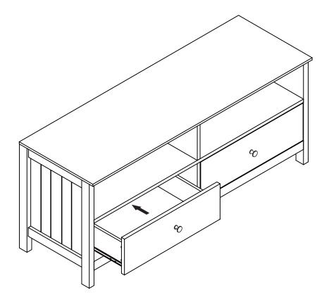
Carefully insert the drawers into the lowline by gently guiding the runners into the tracks.
