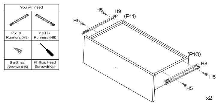
Attach 2 x DL Runners (H8) to the bottom of Left Drawer Sides (P10x2) and 2 x DR Runners (H9) to the bottom of Right Drawer Sides (P11x2) with 8 x Small Screws (H5) by tightening with the Phillips Head Screwdriver.
