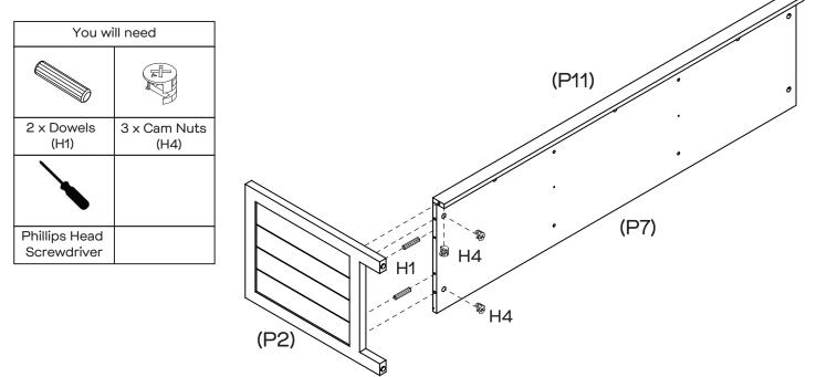
Insert 2 x Dowels (H1) into Left Side Panel (P2) as shown. Insert 3x Cam Nuts (H4) into Rail & Bottom Panel (P11&P7) as shown. Rotate the cam nuts so the arrow points towards the incoming cam bolts. Attach Rail & Bottom Panel (P11&P7) to Left Side Panels (P2) by tightening the Cam Nuts (H4) with the Phillips Head Screwdriver.
