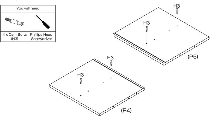
Attach 4 x Cam Bolts (H3) to Dividers (P4&P5) by tightening with the Phillips Head Screwdriver.
