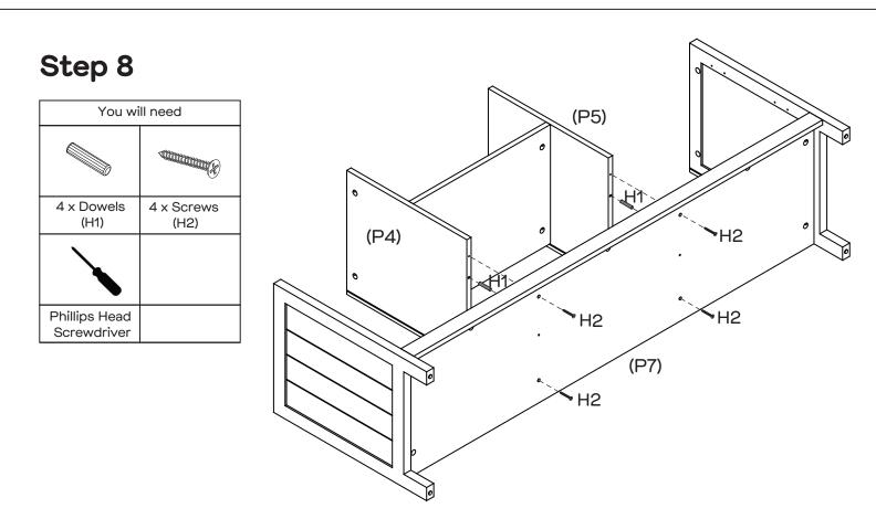
Insert 4 x Dowels (H1) into Bottom Panel (P7) as shown. Attach Dividers (P4&P5) to Bottom Panel (P7) with 4 x Screws (H2) by tightening with the Phillips Head Screwdriver.
