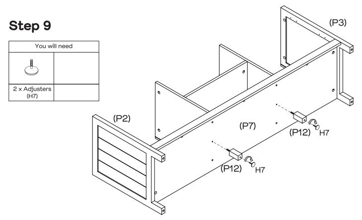
Attach Adjustable Support Legs (P12x2) to Bottom Panel (P7). Attach 2 x Adjusters (H7) to Support Legs (P12x2).
