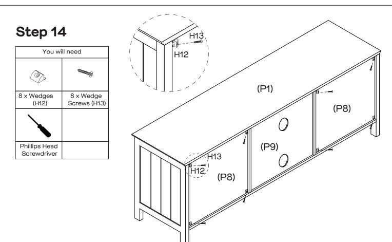
Secure Back Panels (P8 & P9  $\times$  2) in place with 8  $\times$  Wedges (H12) using 8  $\times$  Wedge Screws (H13) by tightening with the Phillips Head Screwdriver.
