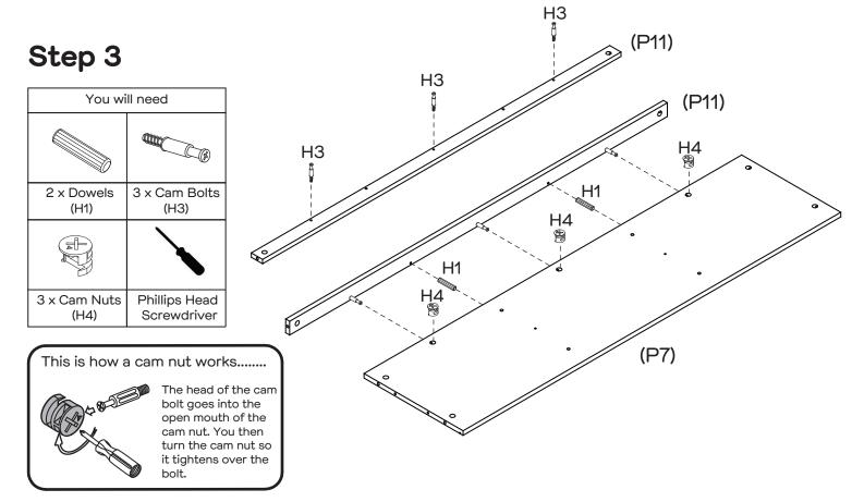
Attach 3 x Cam Bolts (H3) to Rail (P11) by tightening with the Phillips Head Screwdriver. Insert  $2 \times Dowels$  (H1) into Bottom Panel (P7) as shown. Insert  $3 \times Cam$  Nuts (H4) into Bottom Panel (P7) as shown. Rotate the cam nuts so the arrow points towards the incoming cam bolts. Attach Rail (P11) to Bottom Panel (P7) by tightening the Cam Nuts (H4) with the Phillips Head Screwdriver.
