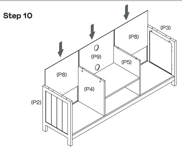
Gently stand the unit upright. Slide Back Panels (P8x2 & P9) into the grooves of Dividers & Left & Right Side Panels (P4 & P5 & P2 & P3).
