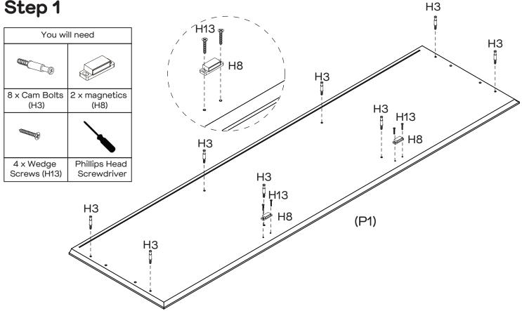
Attach 8 x Cam Bolts (H3) and 2 x Magnetics (H8) to Top Panel (P1) with 4 x Wedge Screws (H13) by tightening with the Phillips Head Screwdriver.
