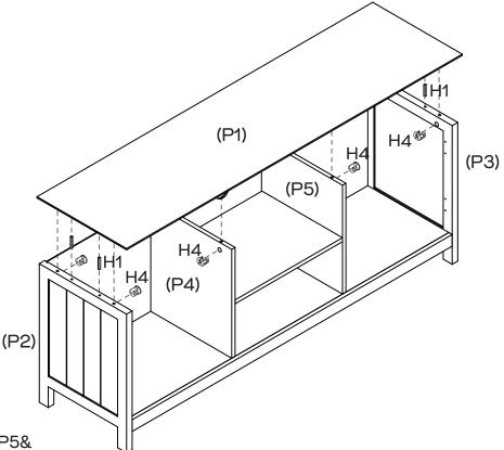
Insert 4 x Dowels (H1) into Left & Right Side Panels (P2&P3) as shown. Insert 8x Cam Nuts (H4) into Dividers & Left & Right Side Panels (P4&P5& P2&P3) as shown. Rotate the
