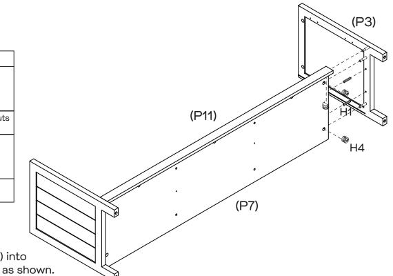
Insert 2 x Dowels (H1) into Right Side Panel (P3) as shown.
