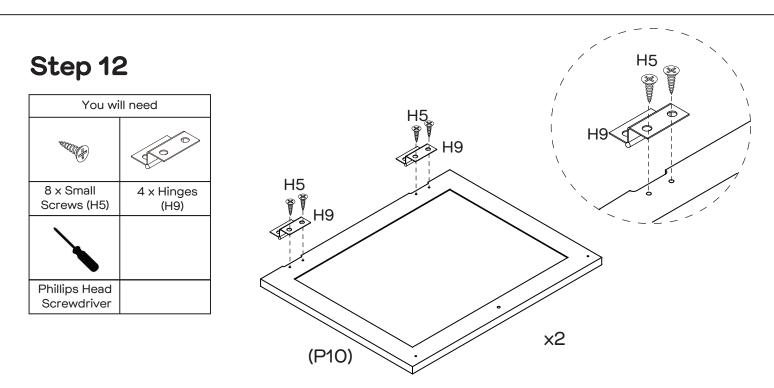
Attach 4 x Hinges (H9) to Doors (P10x2) with 8 x Small Screws (H5) by tightening with the Phillips Head Screwdriver.
