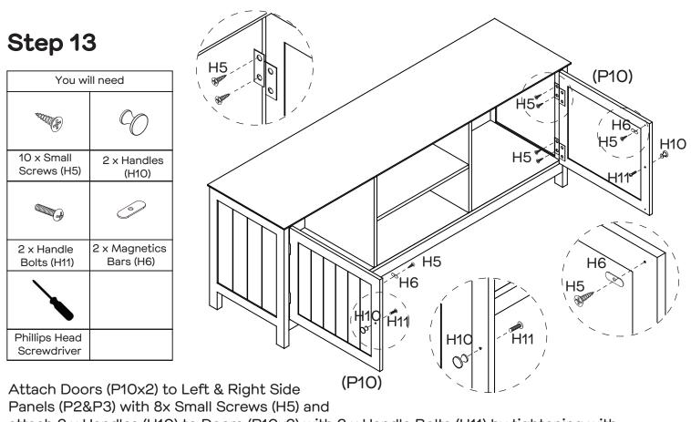
attach 2 x Handles (H10) to Doors (P10x2) with 2 x Handle Bolts (H11) by tightening with the Phillips Head Screwdriver.attach 2 x Magnetics (H6) to Doors (P10x2) with 2 x Small Screws (H5) by tightening with the Phillips Head Screwdriver.
