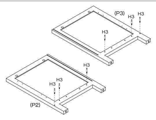
Attach 6 x Cam Bolts (H3) to Left & Right Side Panels (P2&P3) by tightening with the Phillips Head Screwdriver.
