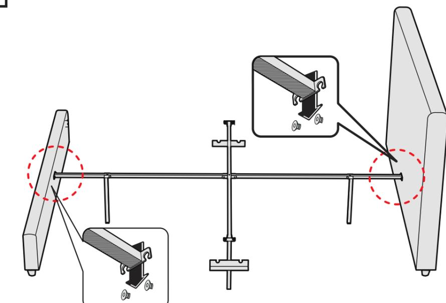
8 ※ To be fully tighten after placing all side rails.
