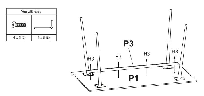
Place rail (P3) under the table top (P1) use screw (H3) to fasten the rail.
