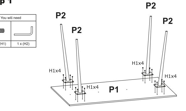
Place legs (P2) on the table top (P1). Use bolts (H1) and allen key (H2) to fasten the legs.
