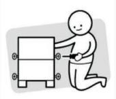
Unless instructed, do not fully tighen screws until the item is fully assembled.
