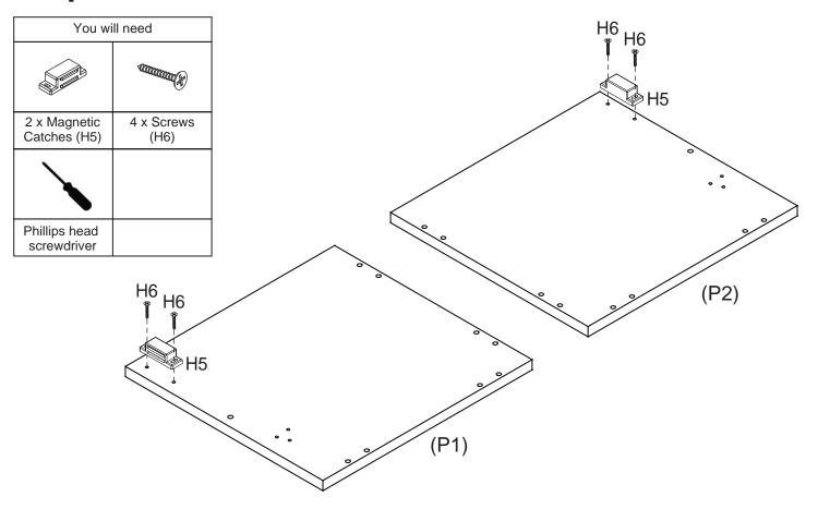
Attach 2 x Magnetic Catches (H5) to Side Panels (P1, P2) with 4 x Screws (H6) as shown.
