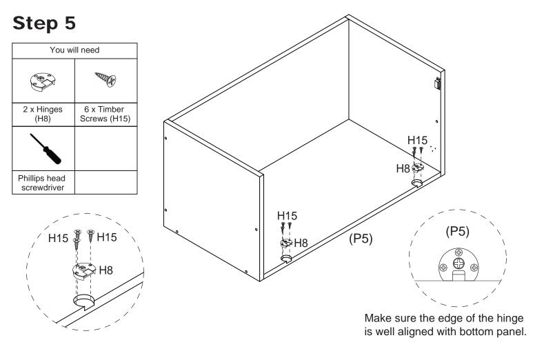
Attach 2 x Hinges (H8) to Bottom Panel (P5) with 6 x Timber Screws (H15). Tighten the screws with a Phillips head screwdriver.
