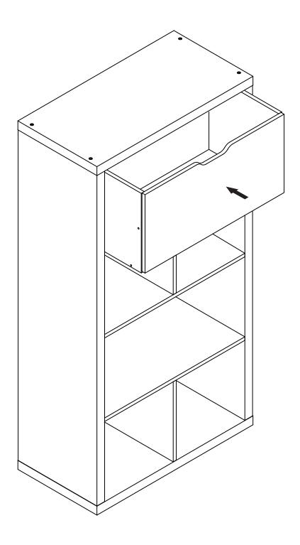
Put the insert cabinet into the bookcase, make sure the door of insert cabinet is flush with the edge of shelf.
