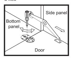
Loosen or tighten the screw indicated a little to adjust the door move up or down a little (see step 3a & Step 3b)
