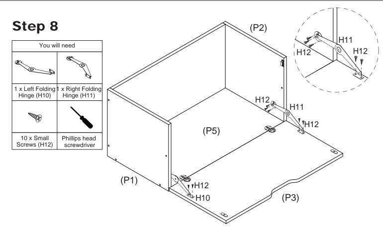
Attach 1 x Left Folding Hinge (H10) and 1 x Right Folding Hinge (H11) to Side Panels (P1, P2) with 6 x Small Screws (H12).
