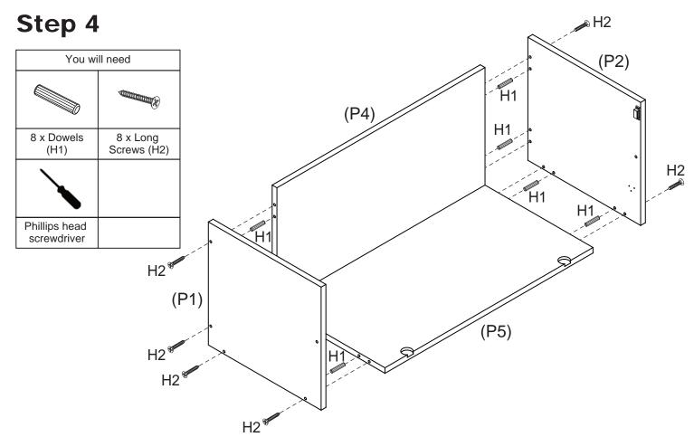
Insert 8 x Dowels (H1) into the holes of Back Panel (P4) and Bottom Panel (P5). Attach Side Panels (P1, P2) to Back Panel (P4) and Bottom Panel (P5) with 8 x Long Screws (H2) using a Phillips head screwdriver.
