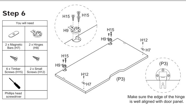
Attach 2 x Magnetic Bars (H7) to Door (P3) with 2 x Small Screws (H12). Attach 2 x Hinges (H9) to Door (P3) with 6 x Timber Screws (H15). Tighten the screws with a Phillips head screwdriver.
