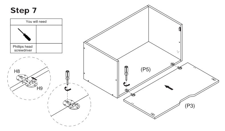
Attach Hinges (H9) to Hinges (H8), if they can't connect, loosen the screw indicated a little. Tighten the screws to connect the hinges on Door (P3) and Bottom Panel (P5).
