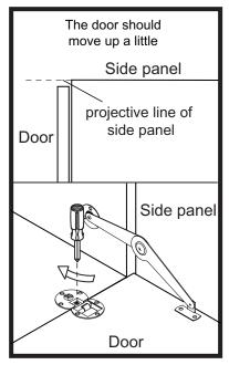
Turn the screw clockwise a little as shown to move door up.
