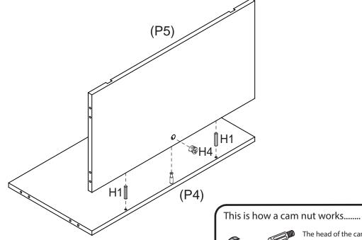
Insert 2 x Dowels (H1) into the holes of Back Panel (P4). Insert 1 x Cam Nut (H4) into the hole of Bottom Panel (P5).
