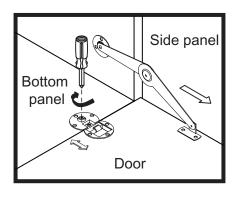
Loosen the screw indicated a little, adjust the hinge to right position (see step 2a & Step 2b), then tighten the screw.
