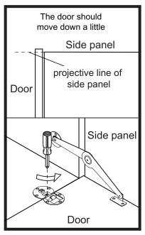
Turn the screw counterclockwise a little as shown to move door down.
