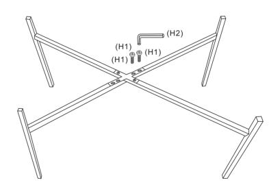
Attach the Leg (P4) with Connector(H3) using Bolts(H1) with Allen Key to tighten. Ensure the leg and connector are level Repeat same way to attach another Leg(P4).
