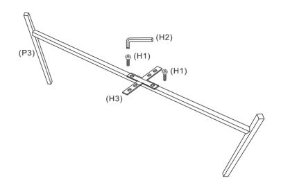
Make sure the connector is in correct position before screwing Attach the Leg (P3) with Connector(H3) using Bolts(H1) with Allen Key to tighten. Ensure the Leg and Connector are level.
