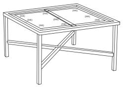
Place the Protectors (H4)onto the frame Place the Glass Top(P1) into the frame
