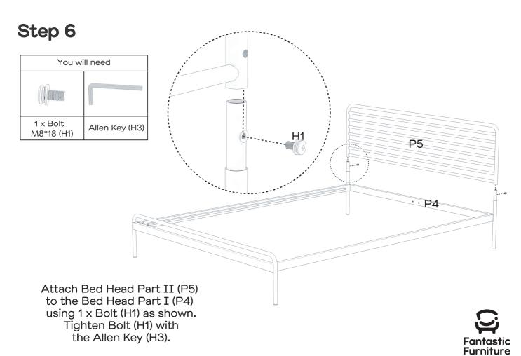
Tighten Bolt (H1) with the Allen Key (H3).
