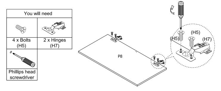
Fix 2 x Hinges (H7) with 4 x Bolts (H5) by using a Phillip head screwdriver.
