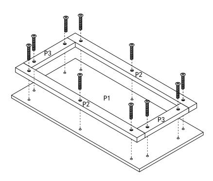
Attach 2 x Long Bottom Rail (P2), 2 x Short Bottom Rails (P3) to Bottom Panel (P1) with 10 x Bolts (H4) by using a Phillips head screwdriver.
