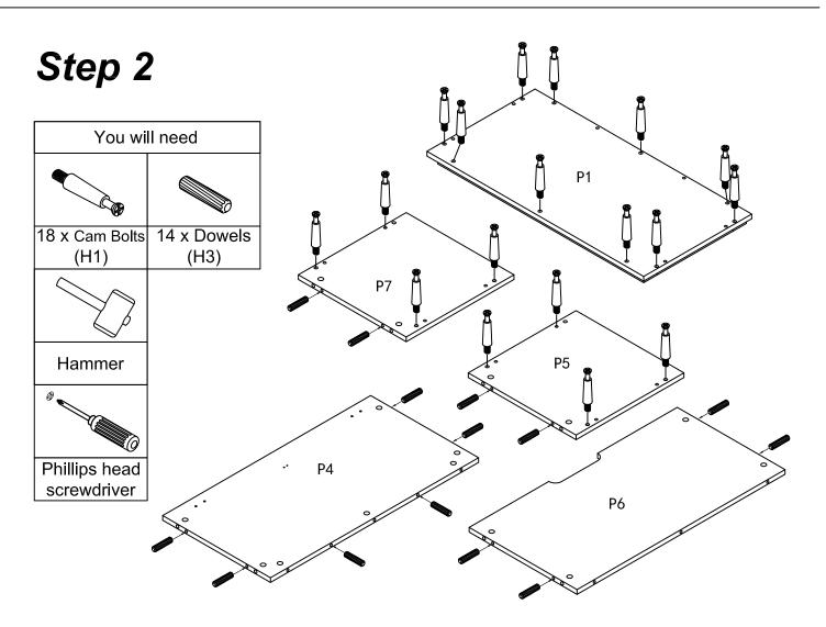
Insert 18 x Cam Bolts (H1) to Panels (P1), (P5) & (P7) and 14 x Dowels (H3) to Panels (P4), (P5), (P6) & (P7) as shown.
