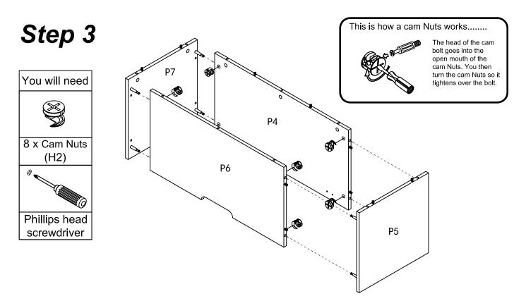
Insert 8 x Cam Nuts (H2) into holes on Back Panel (P4) and Front Panel (P6), rotate the Cam Nuts, so the arrow point towards the incoming Cam Bolts, attach (P5), (P7) to (P6) and (P4) as shown, turn the Cam Nuts clockwise to tighten.
