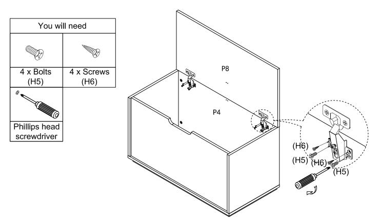
Attach (P8) to the Box Back Panel (P4) with 4 x Bolts (H5) and 4 x Screws (H6) as showing by using a Phillips head screwdriver as showing.
