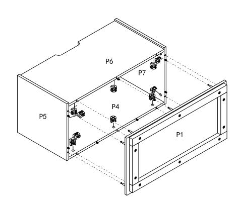
Insert 10 x Cam Nuts (H2) into holes on Panels (P4), (P5), (P6) & (P7), rotate the Cam Nuts, so the arrow points towards the incoming Cam Bolts, then attach (P1) to (P4), (P5), (P6) & (P7) as shown, turn the Cam Nuts clockwise to tighten.
