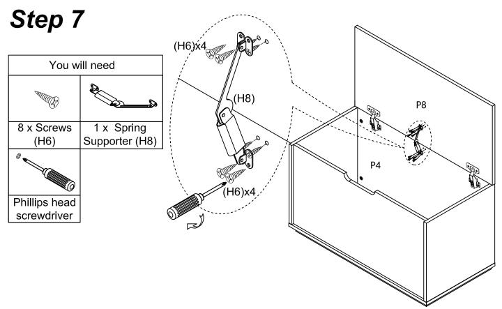
Connecting Back Panel (P4) and Top Panel (P8) with 1 x Spring Supporter (H8) and 8 x Screws (H6) by using a Phillips head screwdriver.
