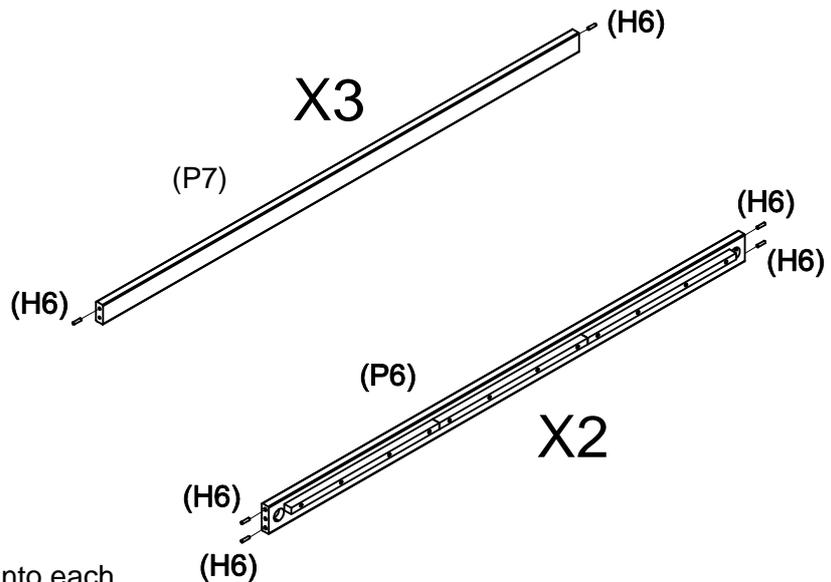
Insert 2 x Wooden Dowels (H6) into each roof bar (P7).
