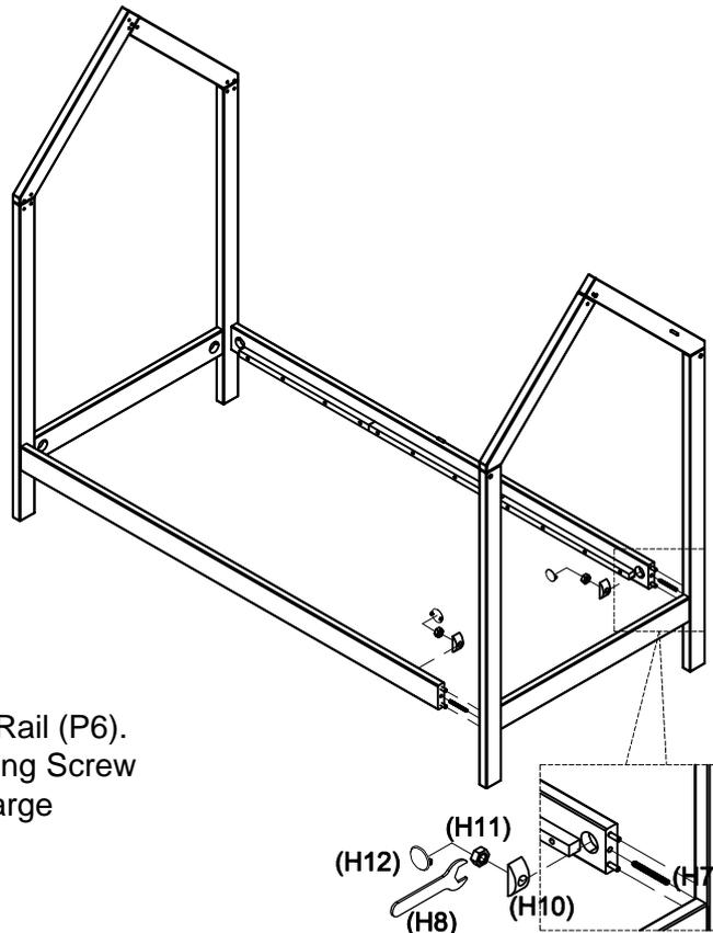
Insert 1 x Locking Pins (H7) to each Side Rail (P6). Insert 1 x Locking Nut (H10) and 1 x Locking Screw (H11), screw the Locking Nuts by using Large Spanner (H8), but don't screw tightly.
