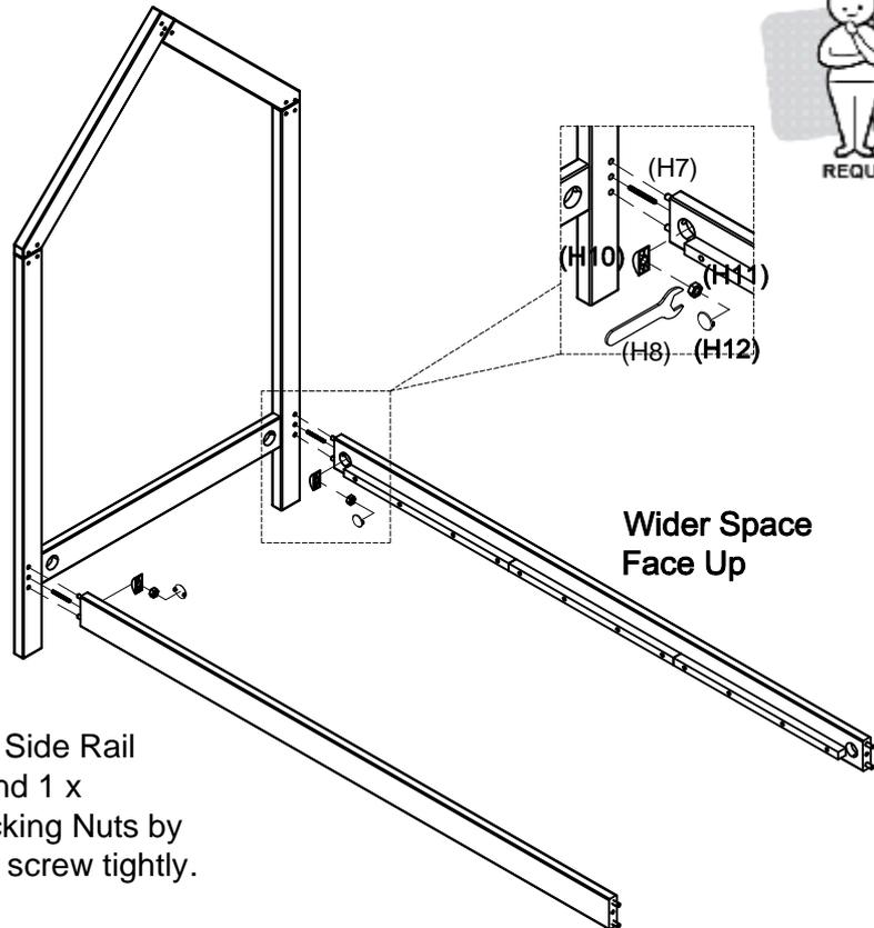
Insert 1 x Locking Pins (H7) to each Side Rail (P6). Insert 1 x Locking Nut (H10) and 1 x Locking Screw (H11), screw the Locking Nuts by using Large Spanner (H8), but don't screw tightly.
