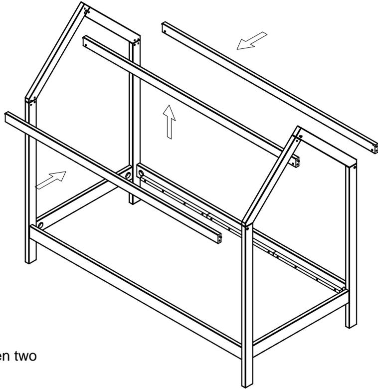
Insert 3 x Roof Bars (P7) between two Sides.
