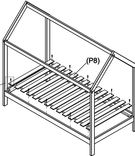
Make sure the inner space of bed frame is square, screw the locking nuts on side rails until tight, put the Slat (P6) on slat holder, use 10 x Wood Screws (H3) to fix the slat. Put 4 x Locking Lids (H12) on opening hole of side rails.
