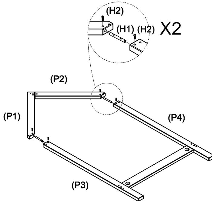
Insert 2 x Steel Dowels (H1) into the Legs and Rails (P1 and P3; P2 and P4). Attach 4 x Bolts (H2) by using a Phillips head screwdriver.
