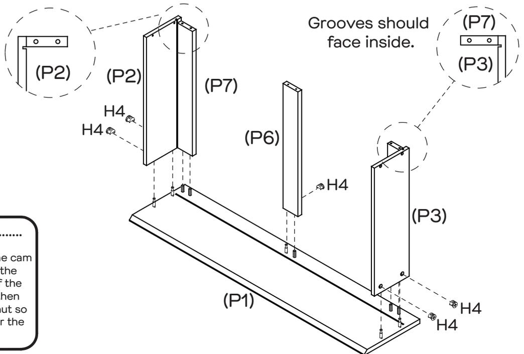
Insert 5 x Small Cam Nuts (H4) into the holes of Drawer Sides (P2, P3) and Central Drawer Support (P6). Rotate the cam nuts so the arrows point towards the incoming cam bolts. Align the holes, and secure Drawer Sides (P2, P3) and Drawer Supports (P6, P7) into place, and then tighten the cam nuts.
