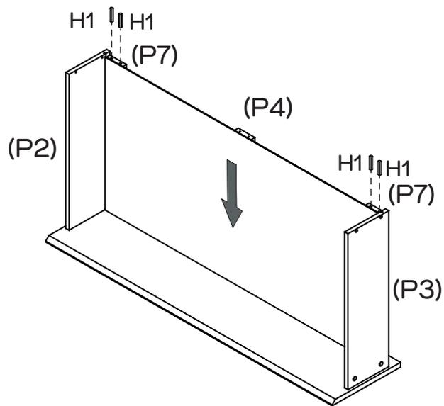
Slide Drawer Base (P4) in through the grooves on Drawer Sides (P2, P3). Insert 4 x Dowels (H1) into Drawer Supports (P7).
