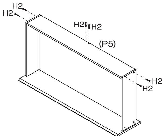
Attach Drawer Back (P5) to Drawer Sides (P2, P3) and Central Drawer Support (P6) with 6 x Long Screws (H2). Make sure that the grooves line up the whole way around the drawer. Repeat Step 1 to Step 5 to assemble the other 3 drawers.
