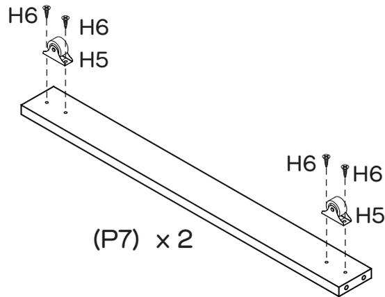
Attach 2 x Wheels (H5) to Drawer Support (P7) with 4 x Small Screws (H6). Repeat Step 2 again with the other Drawer Support (P7).
