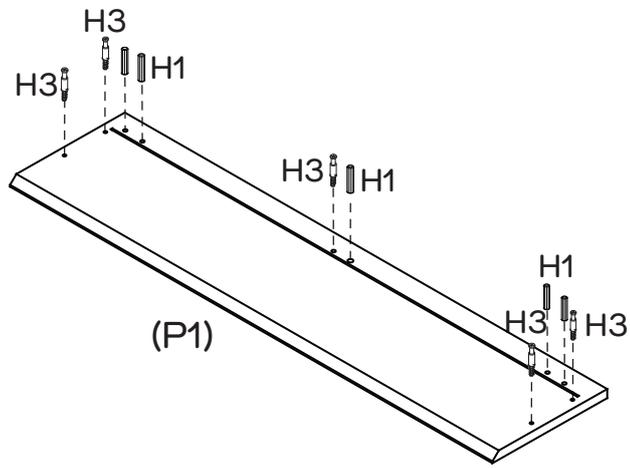
Insert 5 x Dowels (H1) into Drawer Front (P1).
